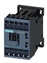
power contactor, AC-3 12 A, 5.5 kW / 400 V 1 NC, 24 V DC 0.85-1.85\*US 3-pole, size S00 spring-type terminal not expandable with auxiliary switch
