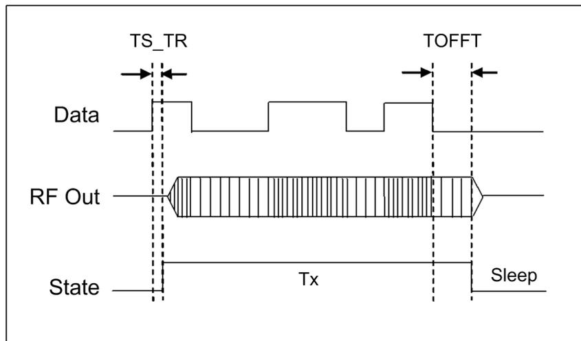
Figure 4. 'Power & Go' Mode: Transmitter Timing Operation
