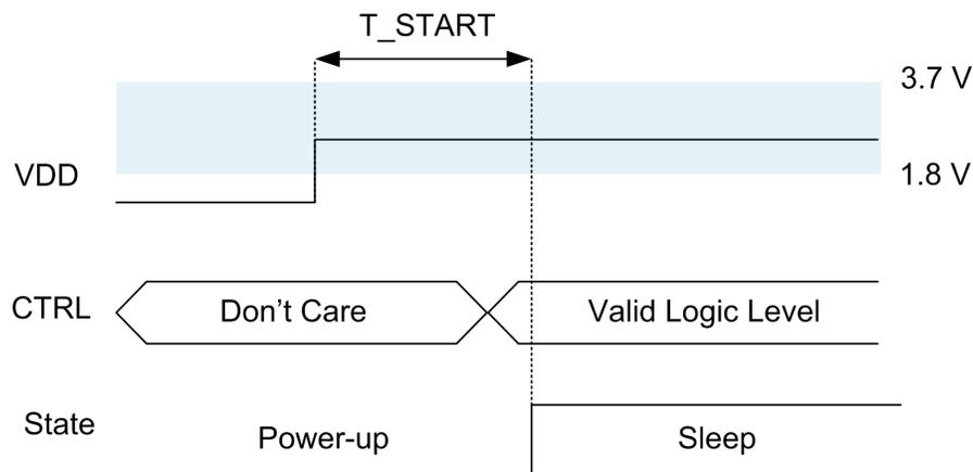
Figure 7. Power-up Timing
