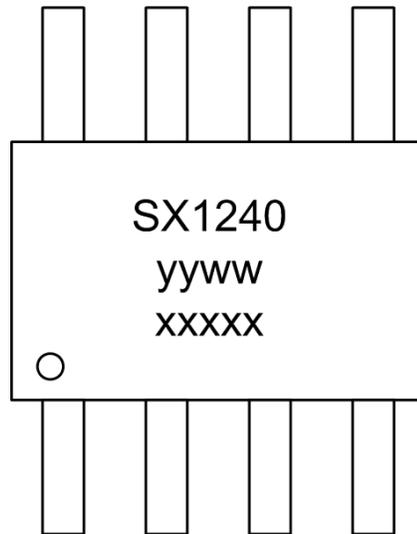
Figure 2. Marking Diagram
