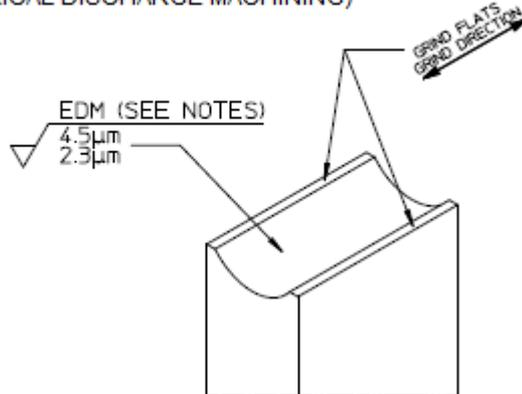
**FIGURE 23: EDM surface finish**
