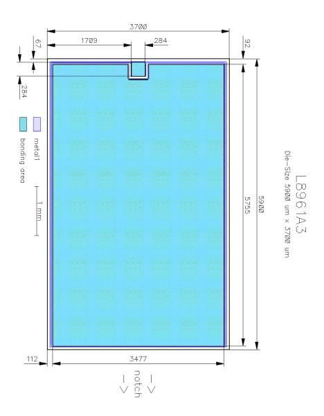
Figure 1 Outline Chip, dimensions in µm
