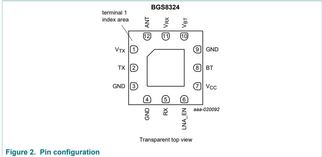
Figure 2. Pin configuration
