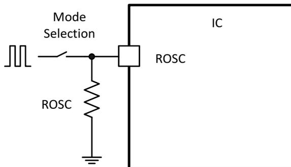
Figure 31. Works With Resistor Mode and Synchronization Mode
