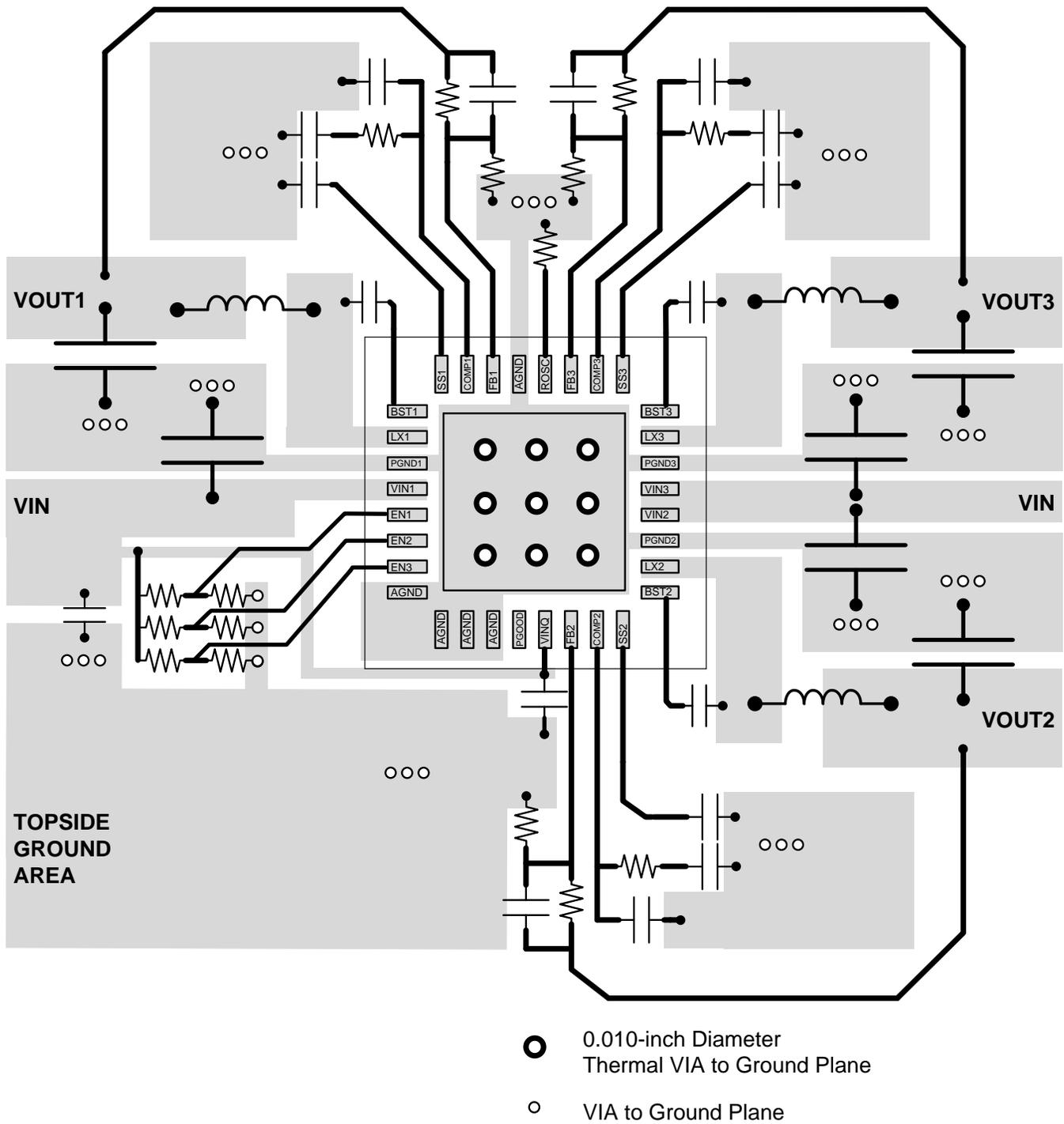
Figure 50. PCB Layout
