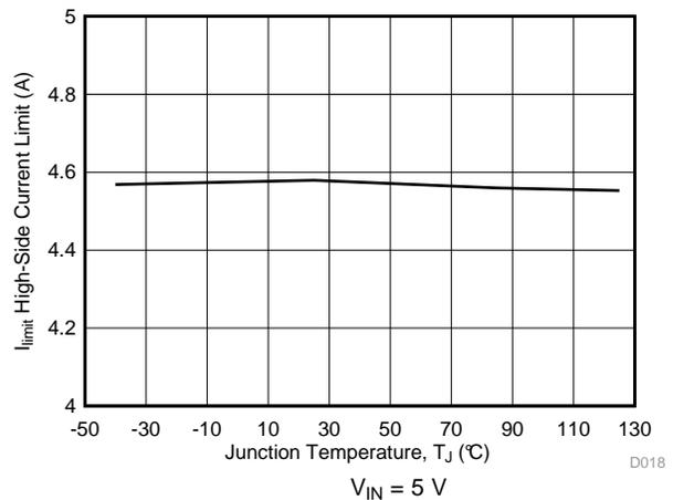
Figure 18. Buck1 High-Side Current Limit vs Temperature
