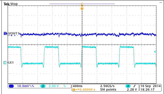
Figure 37. Buck1, Output Voltage Ripple, Iout = 3 A
