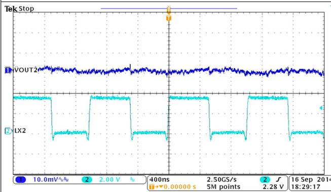
Figure 38. Buck2, Output Voltage Ripple, Iout = 2 A
