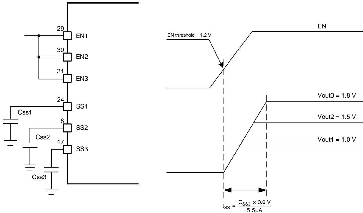
Figure 26. Simultaneous Startup Sequence Using SSx Pins
