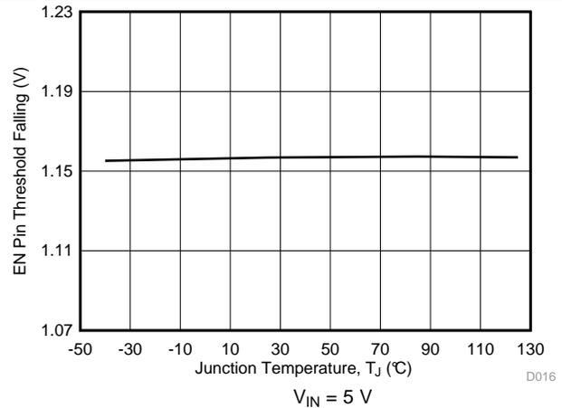
Figure 16. EN Pin Threshold Falling vs Temperature
