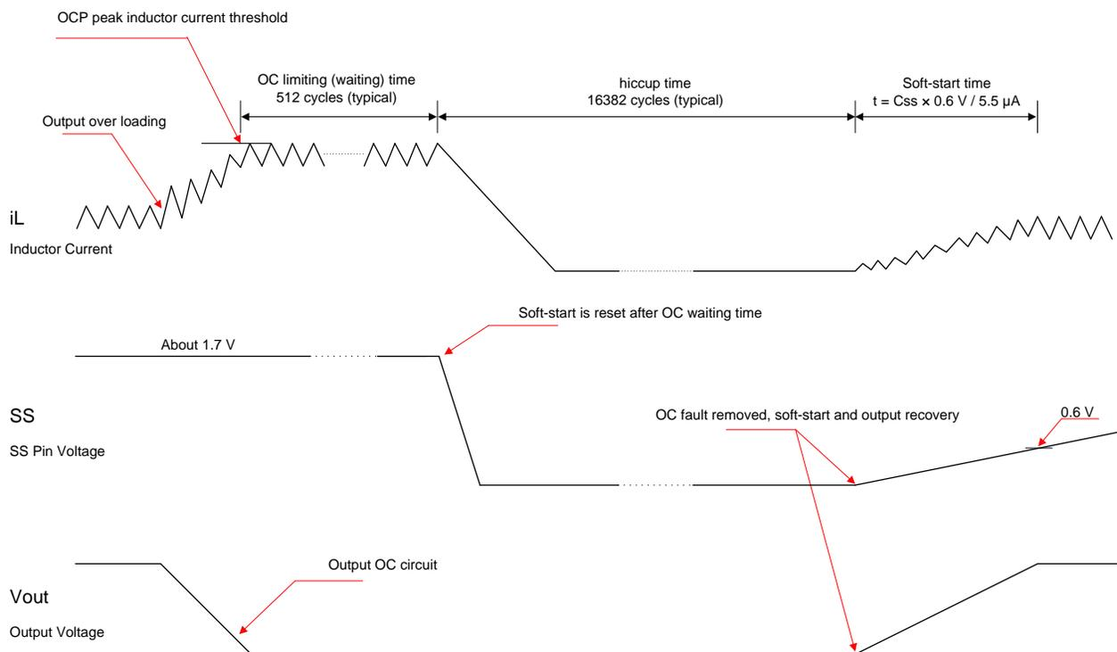
**Figure 29. Overcurrent Protection**
