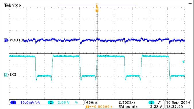
Figure 39. Buck3, Output Voltage Ripple, Iout = 2 A
