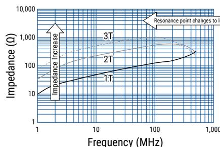
Figure 3 - Effective band range of Nanocrystal core material. (Representative example, measured with same-dimension ring core)
