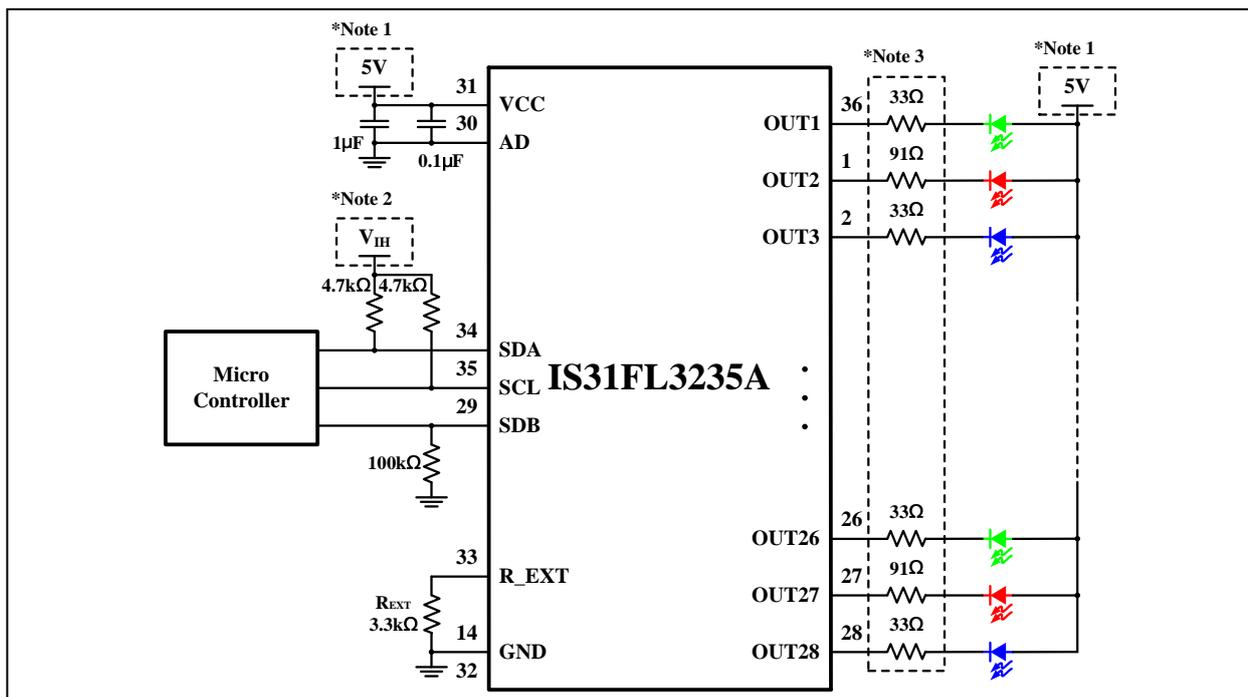
Figure 2 Typical Application Circuit ( $V_{CC}=5V$ )
