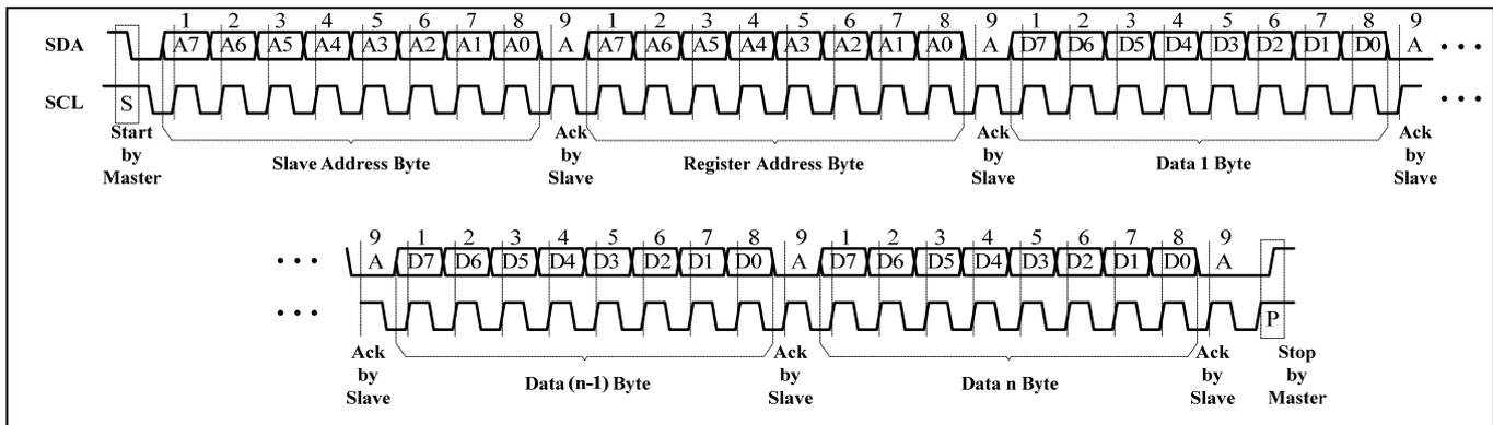
Figure 6 Writing to IS31FL3235A (Automatic Address Increment)
