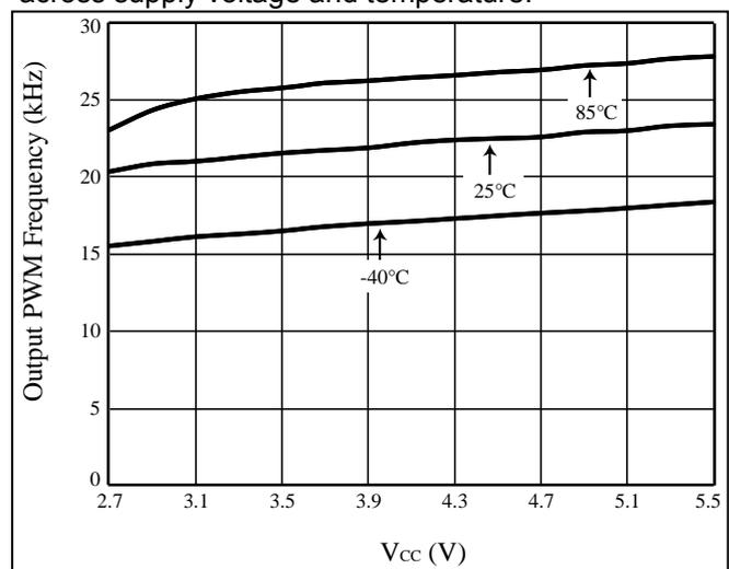
**Figure 9** V<sub>CC</sub> vs. Output PWM Frequency
