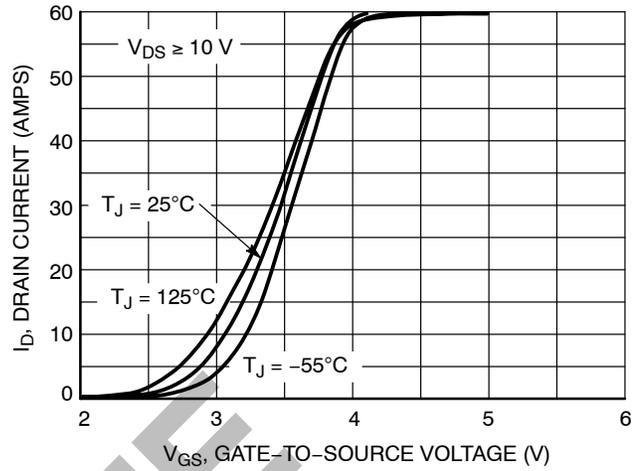
**Figure 2. Transfer Characteristics**
