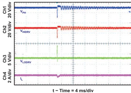
Figure 29. Near 100% Duty Cycle Bootstrap Recharge Pulse
