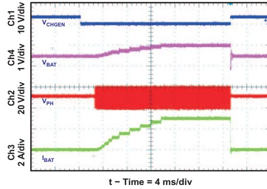
Figure 26. Charge Enable / Disable and Current Soft-Start
