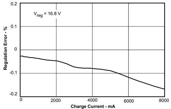
Figure 6. BAT Voltage Regulation Accuracy vs Charge Current
