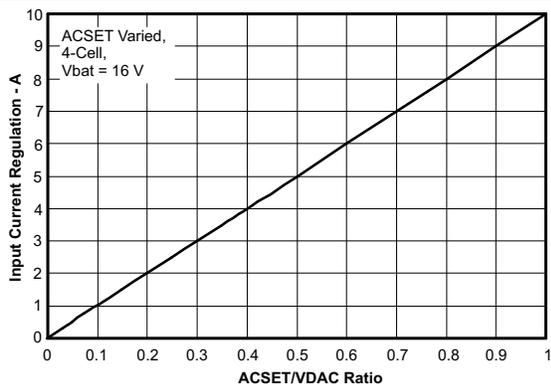
Figure 5. Input Current vs ACSET/VDAC Ratio
