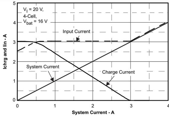
Figure 11. Input Regulation Current (DPM), and Charge Current vs System Current
