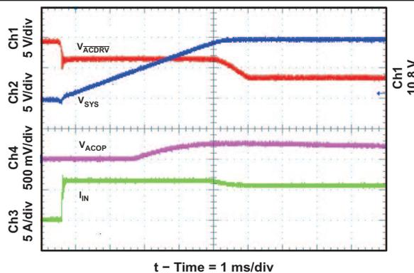
Figure 24. Selector Gate Drive Voltages, 700 ms Delay After ACDET
