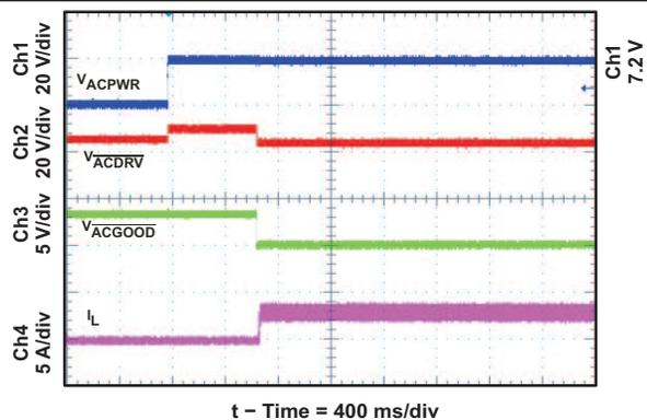
Figure 23. System Selector On Adapter Insertion
