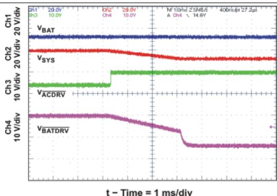
Figure 21. System Selector Learn Turnon With 390 µF SYS-to-PGND System Capacitor
