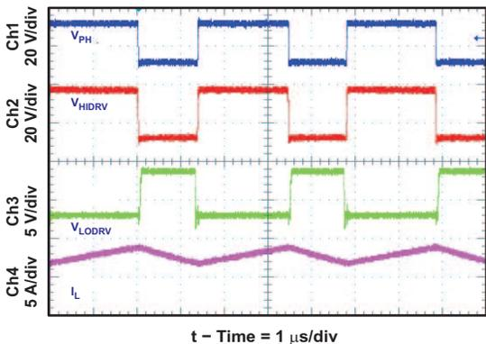
**Figure 31. Continuous Conduction Mode (CCM) Switching Waveforms**
