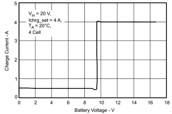
Figure 14. Charge Current Regulation vs BAT Voltage
