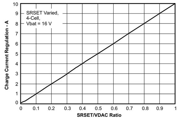
Figure 4. Charge Current vs SRSET/VDAC Ratio
