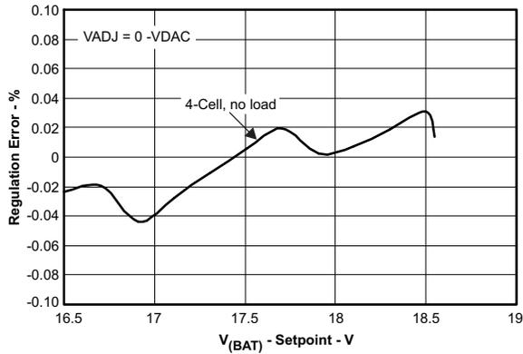
Figure 7. BAT Voltage Regulation Accuracy
