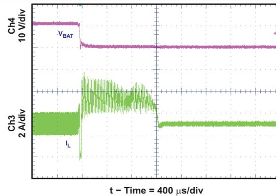
Figure 30. Battery Shorted Charger Response, Overcurrent Protection (OCP) and Charge Current Regulation
