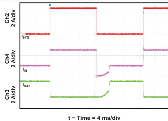
Figure 12. Transient System Load (DPM) Response
