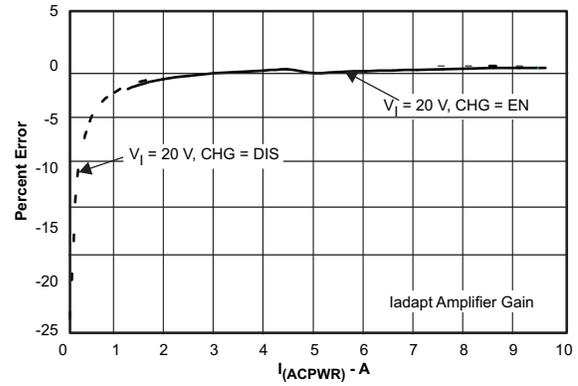
Figure 10. VIADAPT Input Current Sense Amplifier Accuracy
