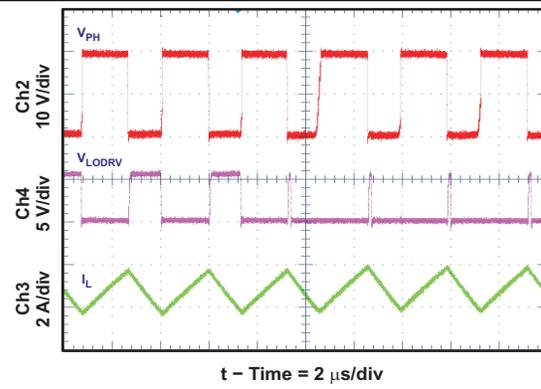
Figure 28. Synchronous to Nonsynchronous Transition
