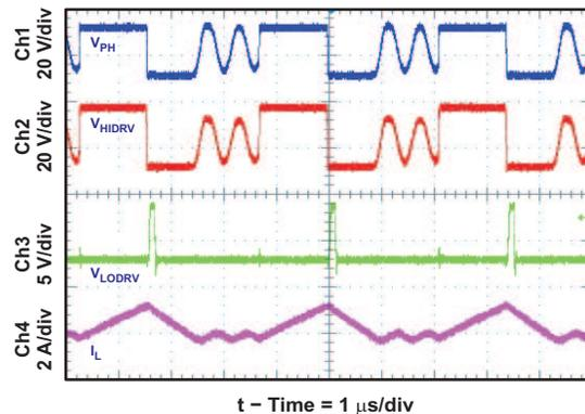
**Figure 32. Discontinuous Conduction Mode (DCM) Switching Waveforms**
