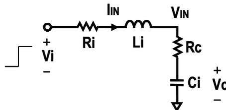
**Figure 38. Simplified Equivalent Circuit During Adapter Insertion**
