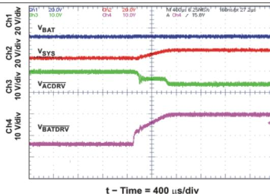
Figure 22. System Selector Learn Turnoff With 390 µF SYS-to-PGND System Capacitor
