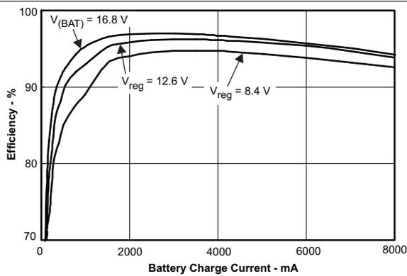
Figure 15. Efficiency vs Battery Charge Current
