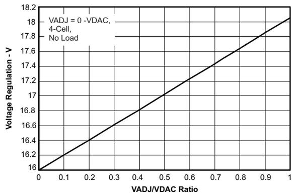
Figure 3. BAT Voltage vs VADJ/VDAC Ratio
