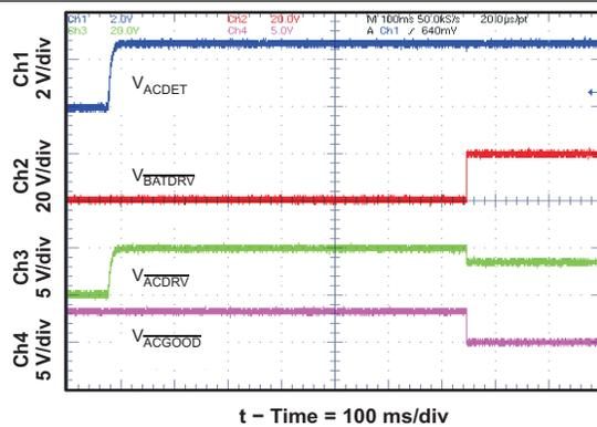
Figure 17. ACDRV and BATDRV Startup
