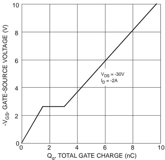
Figure 11 Gate-Charge Characteristics
