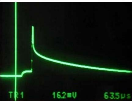
Figure 5. Clamp over shoot (at pulse output); horizontal scale =  $50\mu$ S/div, vertical scale = 50mV/div, supply voltage = 4.5V, clamp over shoot = 162mV.
