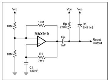
Figure 1. This reset circuit consumes less than 1μA and delivers a 100-μsec-wide reset pulse every 1.3 sec.
