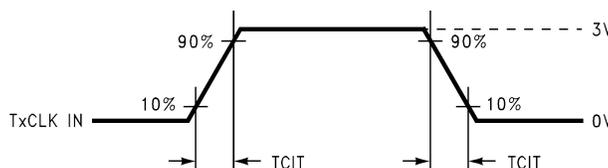
Figure 6. DS90CF363B (Transmitter) Input Clock Transition Time
