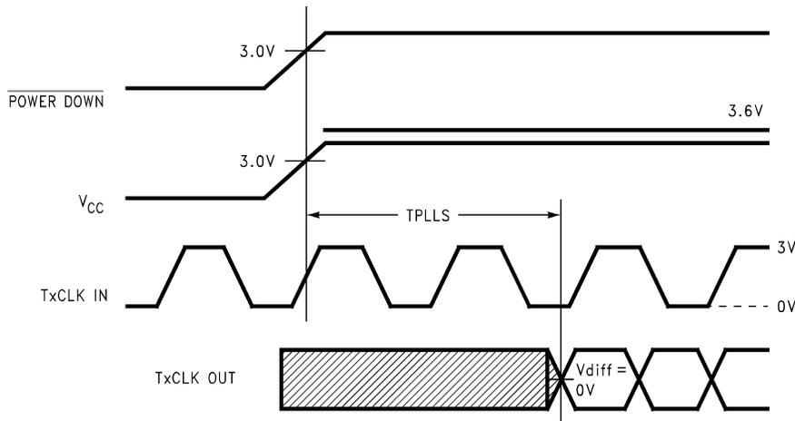
Figure 9. DS90CF363B (Transmitter) Phase Lock Loop Set Time
