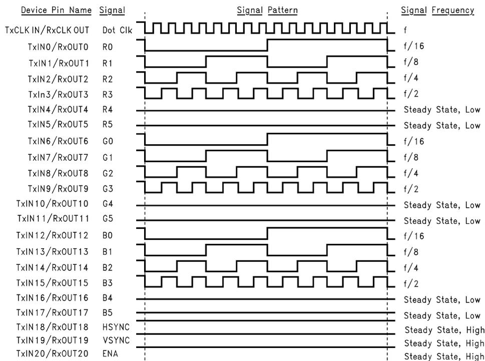
The worst case test pattern produces a maximum toggling of digital circuits, LVDS I/O and CMOS/TTL I/O.
