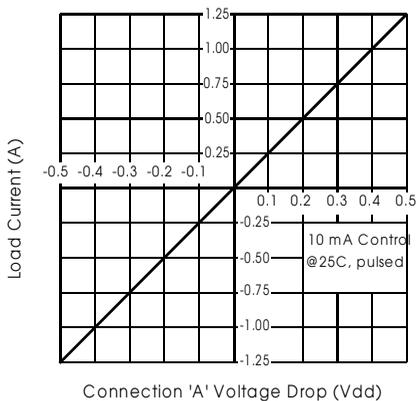
**Figure 3. Linearity Characteristics**
