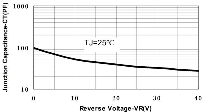
Fig.1-Typical Junction Capacitance
