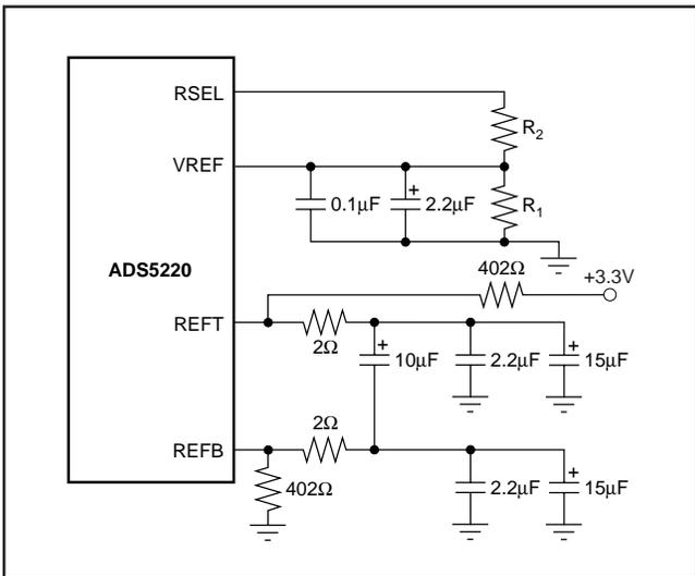
FIGURE 9. Internal Reference Mode for  $V_{REF} = 0.5 \cdot (1 + R_2/R_1)$ .
