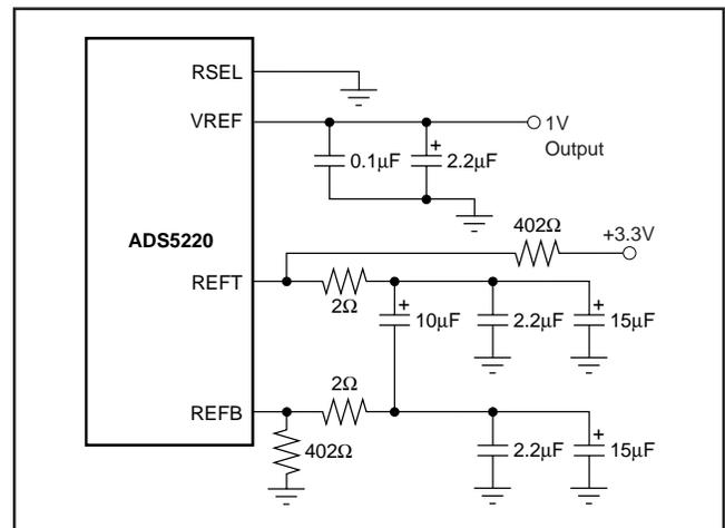
FIGURE 7. Internal Reference Mode for  $V_{REF} = 1V$ .
