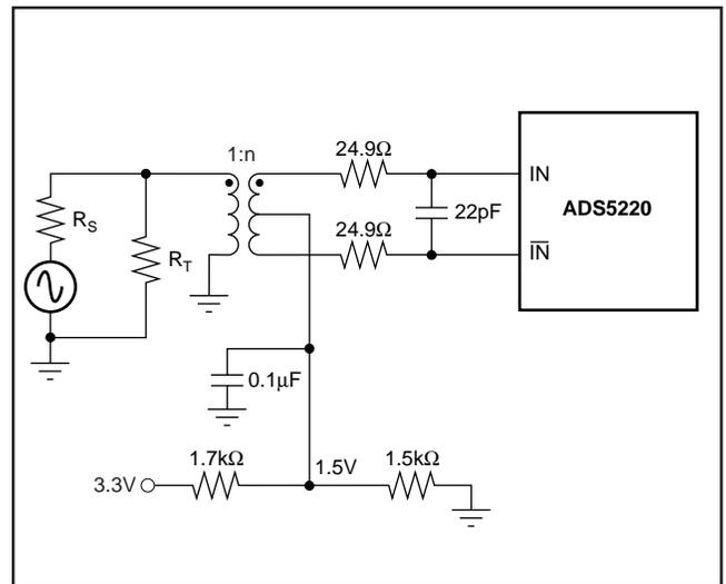
FIGURE 3. Transformer-Coupled Differential Input Configuration of ADS5220.
