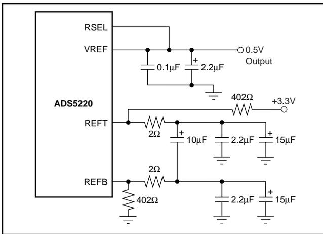
FIGURE 8. Internal Reference Mode for  $V_{REF} = 0.5V$ .
