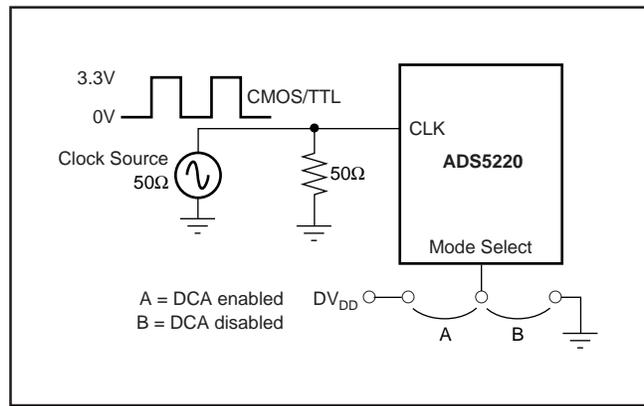
FIGURE 6. General Input Clock Interface of ADS5220.
