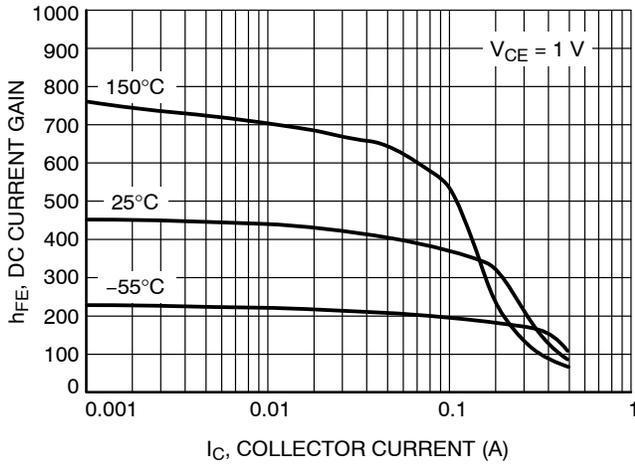
Figure 17. DC Current Gain vs. Collector Current
