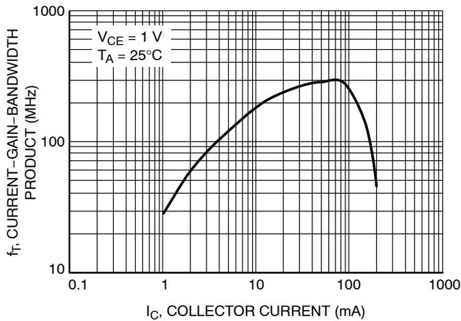
Figure 21. Current Gain Bandwidth Product vs. Collector Current
