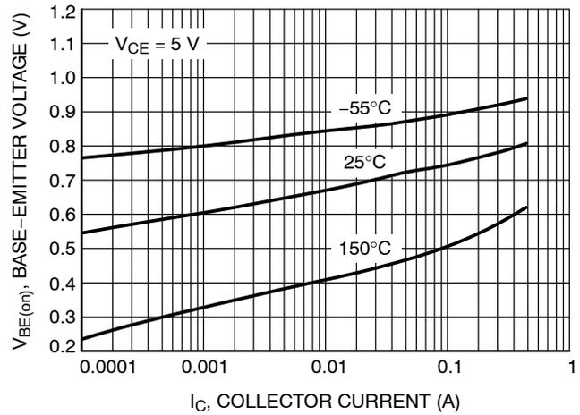
Figure 12. Base Emitter Voltage vs. Collector Current
