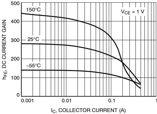
Figure 9. DC Current Gain vs. Collector Current
