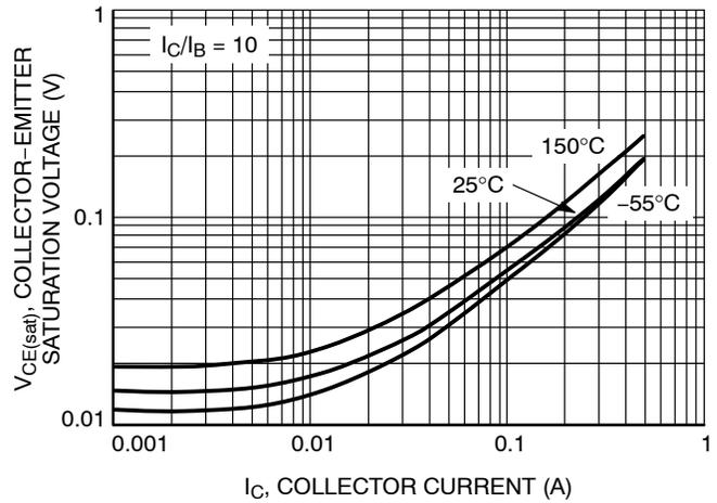
Figure 18. Collector Emitter Saturation Voltage vs. Collector Current
