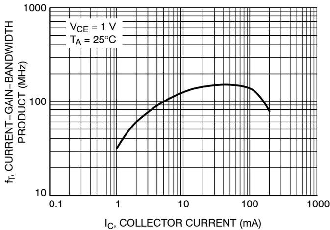
Figure 13. Current Gain Bandwidth Product vs. Collector Current
