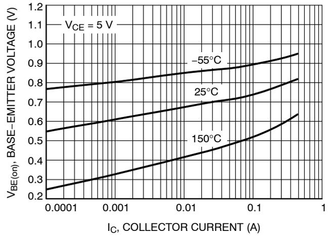
Figure 4. Base Emitter Voltage vs. Collector Current
