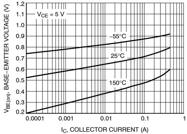
Figure 20. Base Emitter Voltage vs. Collector Current
