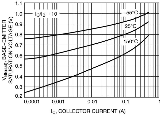
Figure 19. Base Emitter Saturation Voltage vs. Collector Current
