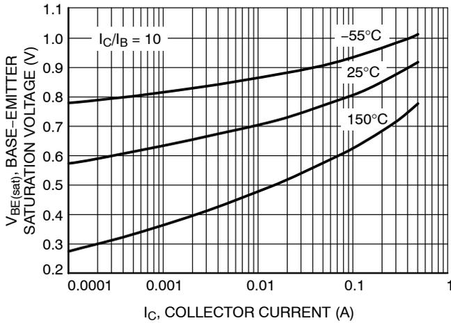
Figure 11. Base Emitter Saturation Voltage vs. Collector Current
