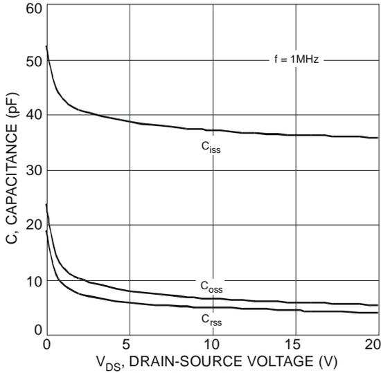
Fig. 9 Typical Capacitance
