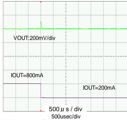
$V_{IN}=5.0V$ ,  $V_{OUT}=3.3V$ , MODE/SYNC= $V_{IN}$  (PWM/PFM automatic switching control),  $T_{opr}=25^\circ C$
