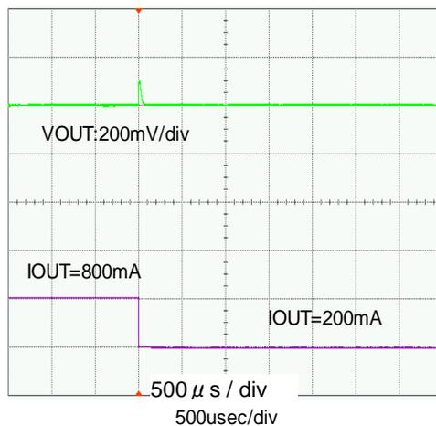
$V_{IN}=5.0V$ ,  $V_{OUT}=3.3V$ , MODE/SYNC=0V (PWM/PFM automatic switching control)
