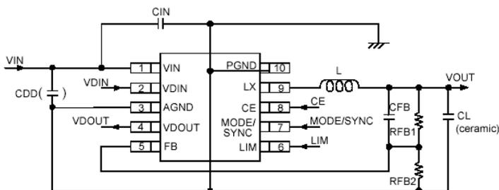
(\*1) A capacitor of 2200pF~0.1 μF is recommended to place at the C<sub>DD</sub> between the AGND pin and the V<sub>DD</sub> pin.
