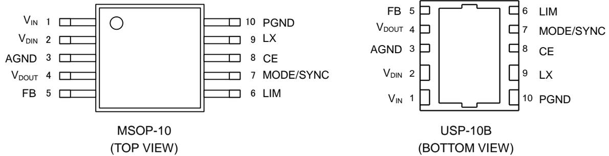
\* For mounting intensity and heat dissipation, please refer to recommended mounting pattern and recommended metal mask when soldering the pad of USP-10B. Mounting should be connected to the GND (No.3,10) pin.
