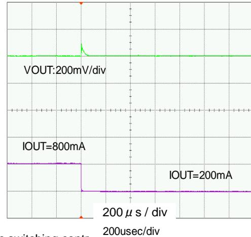
$V_{IN}=5.0V$ ,  $V_{OUT}=1.5V$ ,  $I_C=0V$  (PWM/PFM automatic switching control)
