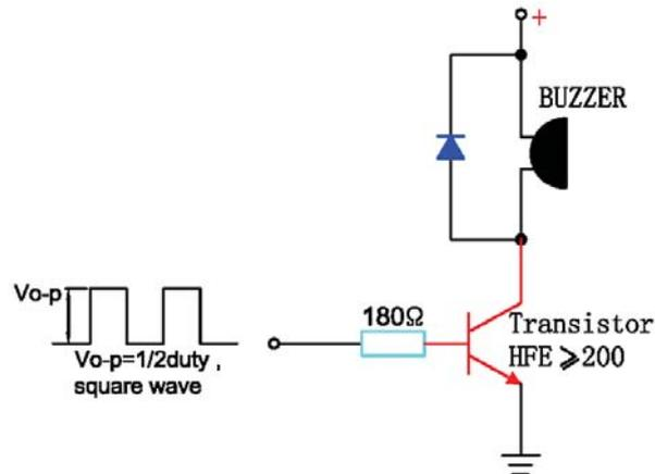
The base current  $I_b$  should be high enough so that it saturates the collector current of the transistor with the CB load.
