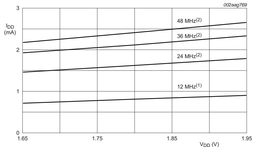
Conditions:  $T_{amb} = 25^\circ\text{C}$ ; Sleep mode entered from flash; all peripherals disabled in the SYSAHBCLKCTRL register (SYSAHBCLKCTRL = 0x1F); all peripheral clocks disabled; internal pull-up resistors disabled.
