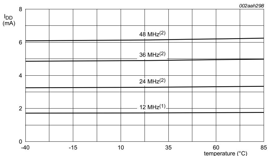
Conditions:  $V_{DD} = 1.8\text{ V}$ ; active mode entered executing code while(1){ } from flash; all peripherals disabled in the SYSAHBCLKCTRL register (SYSAHBCLKCTRL = 0x1F); all peripheral clocks disabled; internal pull-up resistors disabled.
