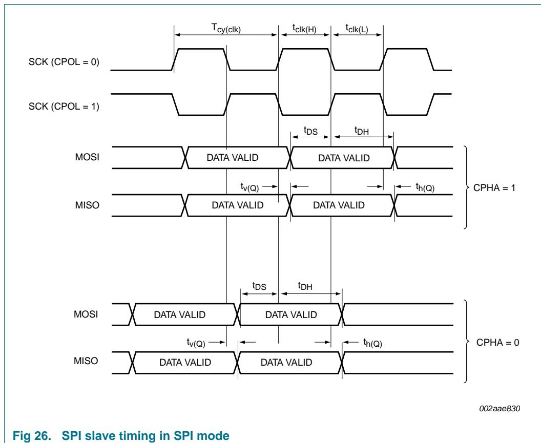
Fig 26. SPI slave timing in SPI mode
