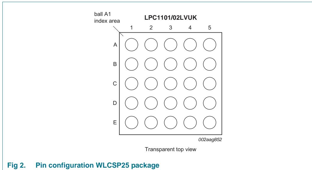
Fig 2. Pin configuration WLCSP25 package
