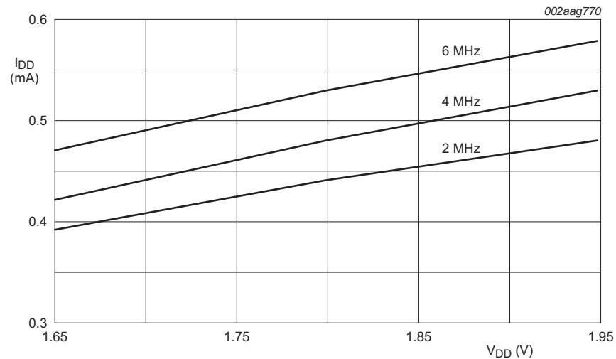
Conditions:  $T_{amb} = 25^\circ\text{C}$ ; Sleep mode entered from flash; all peripherals disabled in the SYSAHBCLKCTRL register (SYSAHBCLKCTRL = 0x1F); all peripheral clocks disabled; internal pull-up resistors disabled; System oscillator and system PLL disabled; IRC disabled; system clock provided by external clock.
