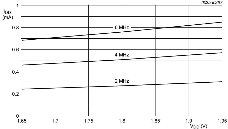
Conditions:  $T_{amb} = 25^\circ\text{C}$ ; active mode entered executing code while(1){ } from flash; all peripherals disabled in the SYSAHBCLKCTRL register (SYSAHBCLKCTRL = 0x1F); all peripheral clocks disabled; internal pull-up resistors disabled; System oscillator, system PLL, IRC, BOD disabled; system clock provided by external clock.
