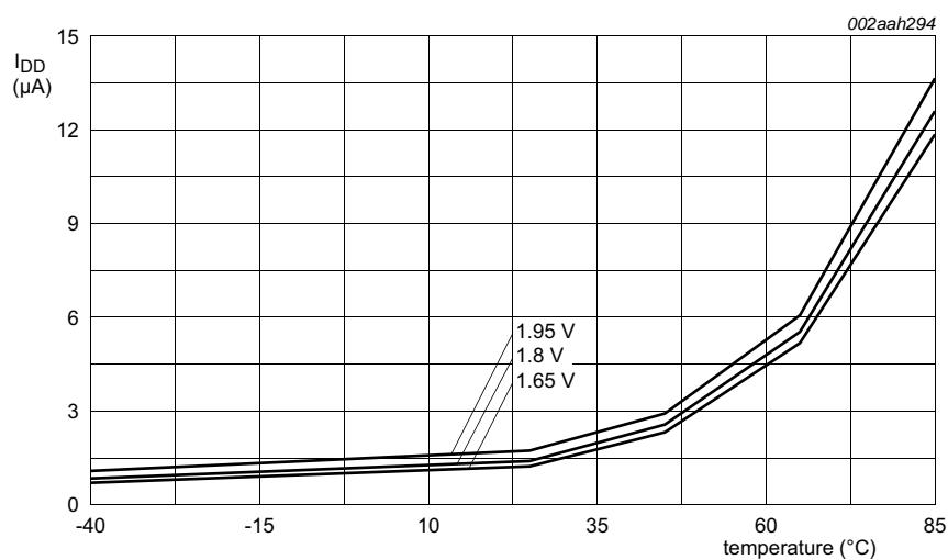
Conditions: all oscillators and analog blocks disabled in the PDSLEEPREG register (PDSLEEPREG = 0x0000 18FF).
