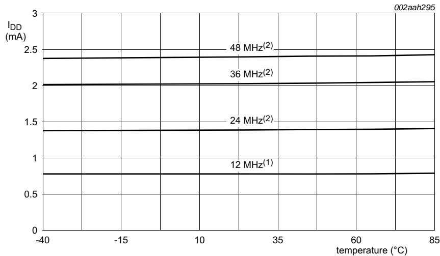
Conditions:  $T_{\text{amb}} = 25 \text{ }^{\circ}\text{C}$ ;  $V_{DD} = 1.8 \text{ V}$ ; Sleep mode entered from flash; all peripherals disabled in the SYSAHBCLKCTRL register (SYSAHBCLKCTRL = 0x1F); all peripheral clocks disabled; internal pull-up resistors disabled.
