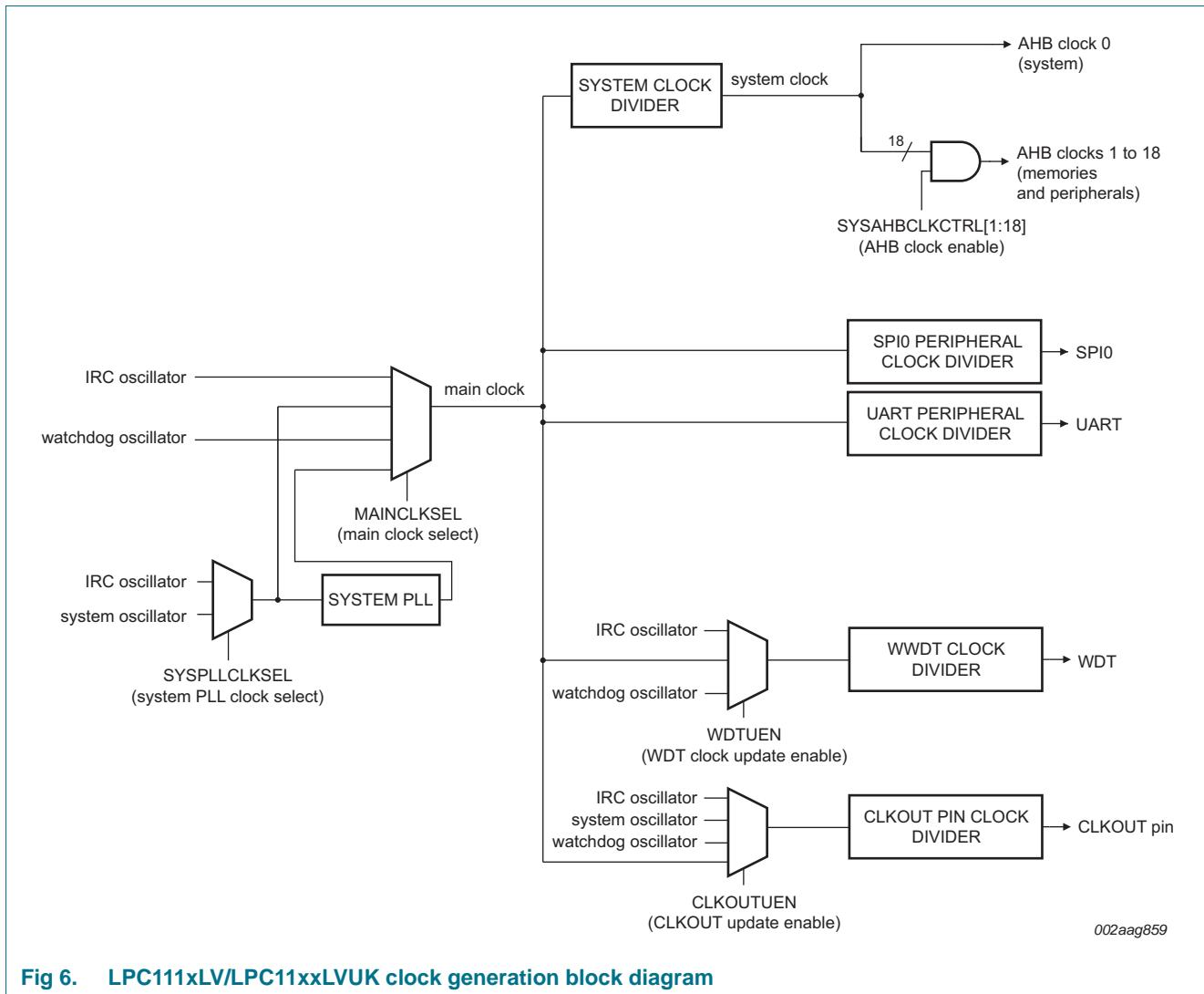
Fig 6. LPC111xLV/LPC11xxLVUK clock generation block diagram
