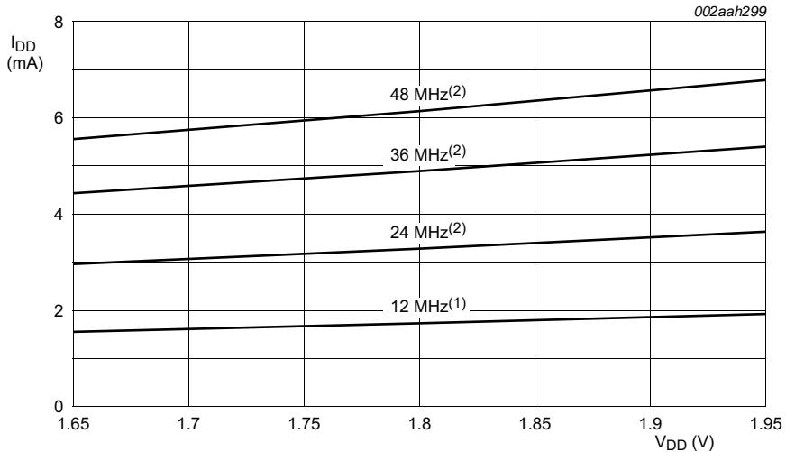
Conditions:  $T_{amb} = 25^{\circ}\text{C}$ ; active mode entered executing code while(1){ } from flash; all peripherals disabled in the SYSAHBCLKCTRL register (SYSAHBCLKCTRL = 0x1F); all peripheral clocks disabled; internal pull-up resistors disabled.
