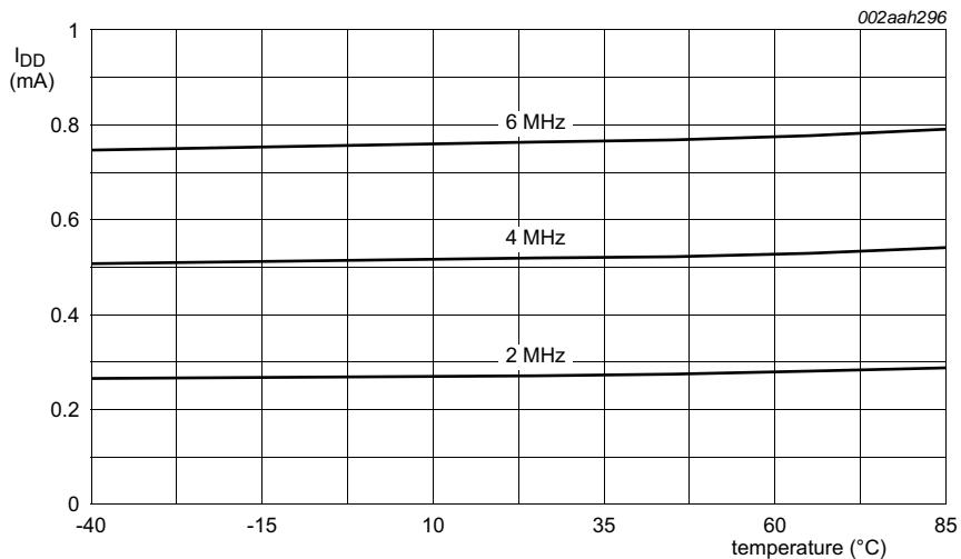
Conditions:  $V_{DD} = 1.8$  V; active mode entered executing code while(1){ } from flash; all peripherals disabled in the SYSAHBCLKCTRL register (SYSAHBCLKCTRL = 0x1F); all peripheral clocks disabled; internal pull-up resistors disabled; System oscillator, system PLL, IRC, BOD disabled; system clock provided by external clock.
