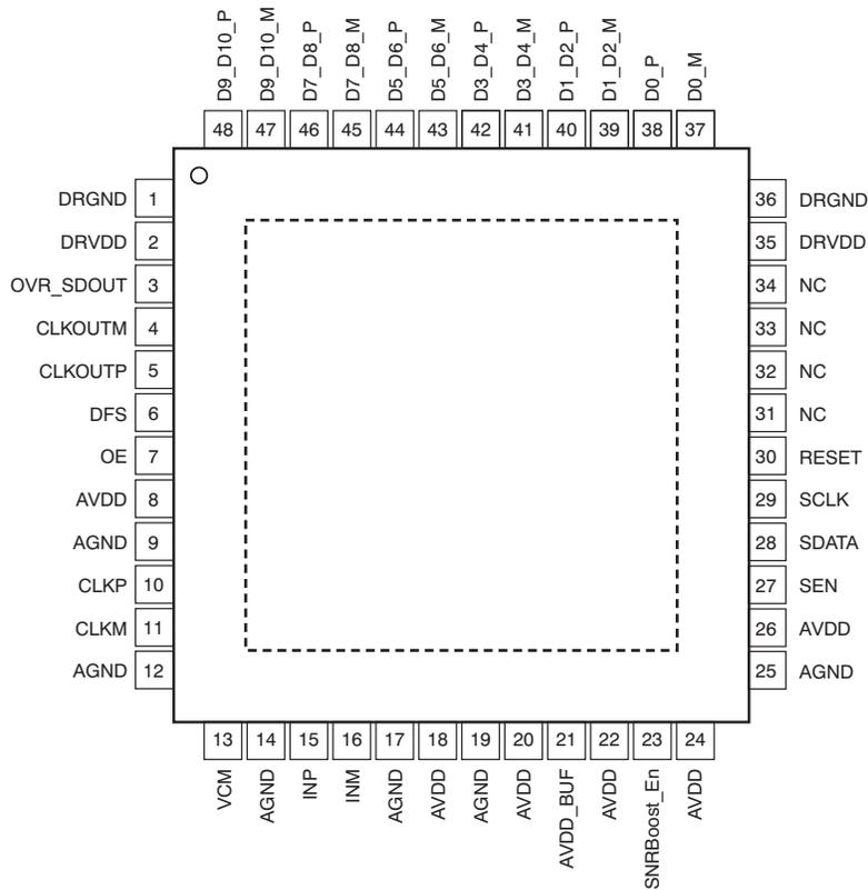
(1) The PowerPAD™ is connected to DRGND.
