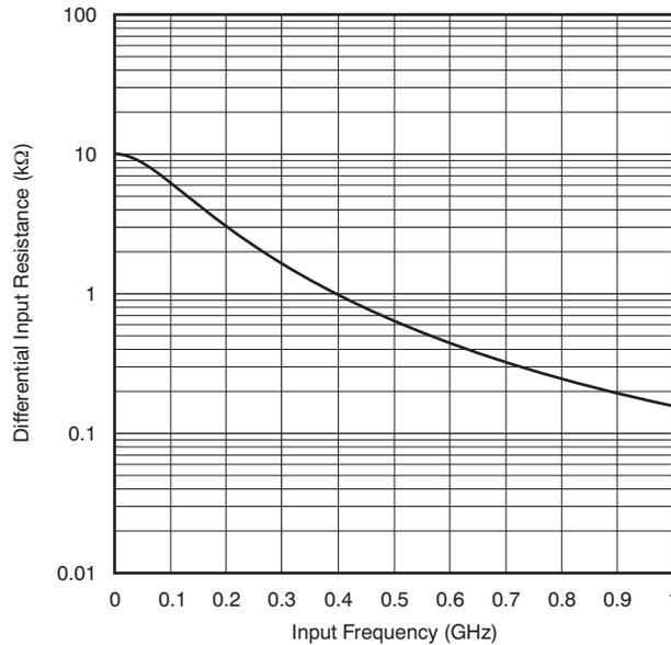
**Figure 59. ADC Analog Input Resistance ( $R_{IN}$ ) Across Frequency**
