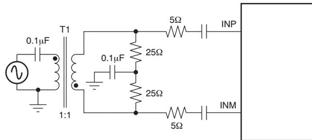
**Figure 61. Drive Circuit for Low Input Frequencies**
