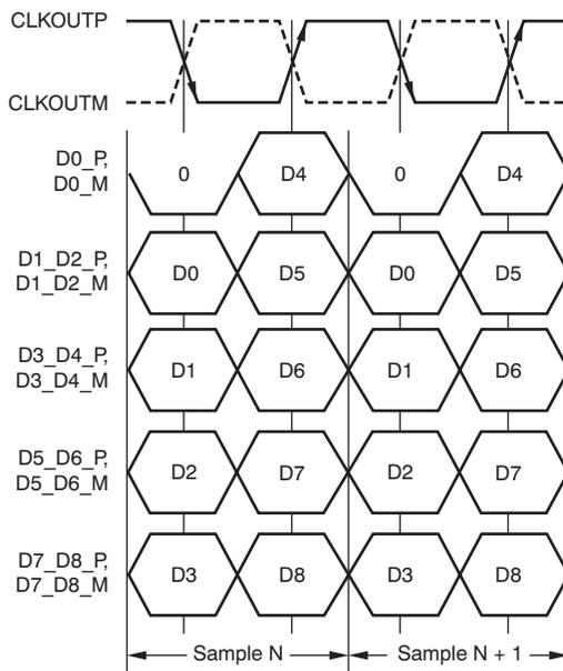
Figure 71. ADS58B19 Byte-Wise Sequence (Only with DDR LVDS Interface)
