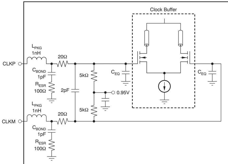
NOTE:  $C_{EQ}$  is 1pF to 3pF and is the equivalent input capacitance of the clock buffer.
