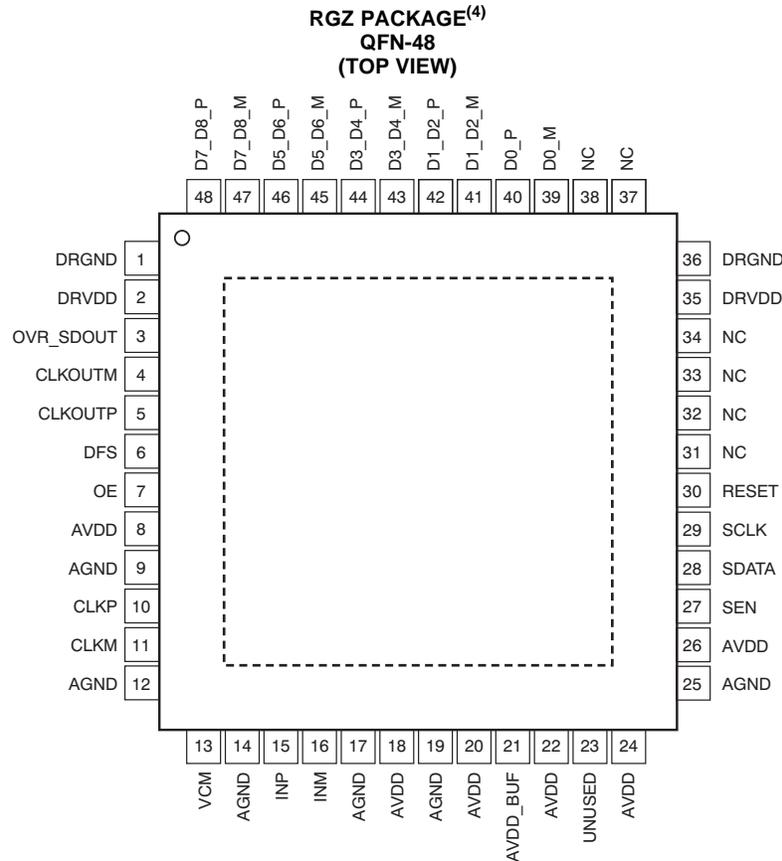
(2) The PowerPAD is connected to DRGND.
