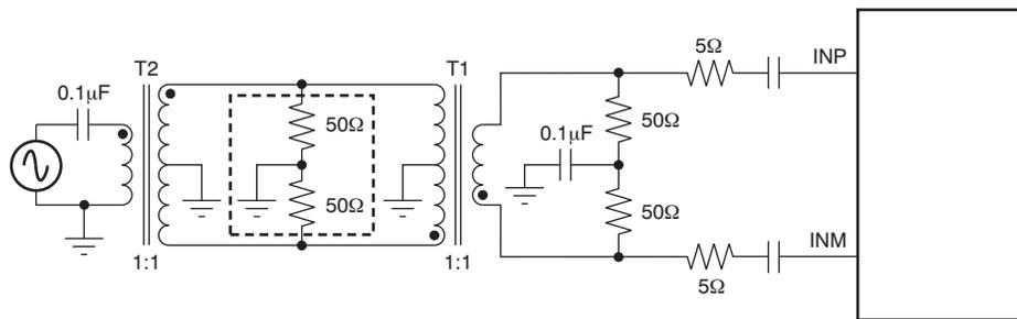
**Figure 62. Drive Circuit for High Input Frequencies**
