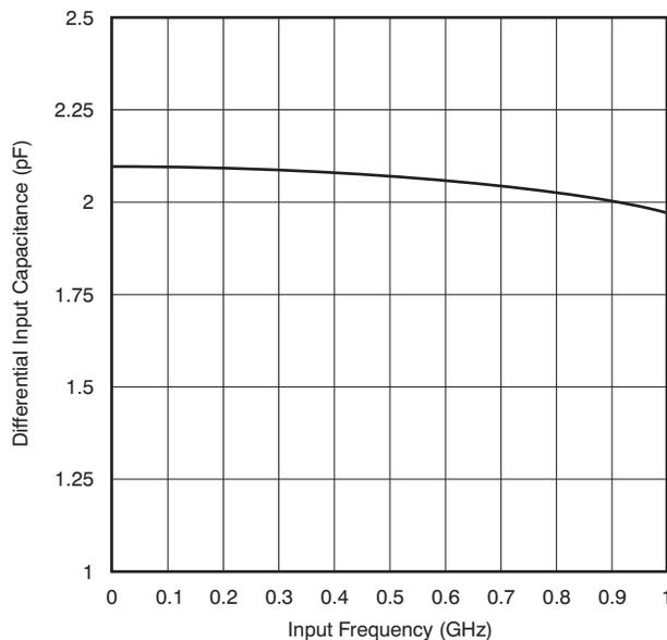
**Figure 60. ADC Analog Input Capacitance ( $C_{IN}$ ) Across Frequency**
