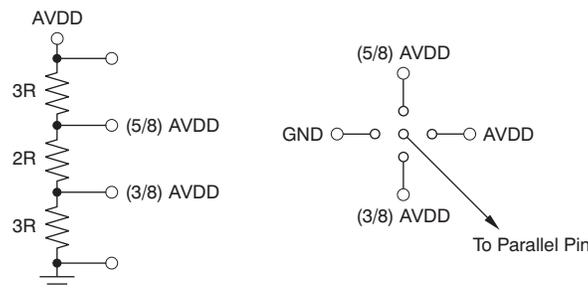
**Figure 11. Simplified Diagram to Configure DFS Pin**
