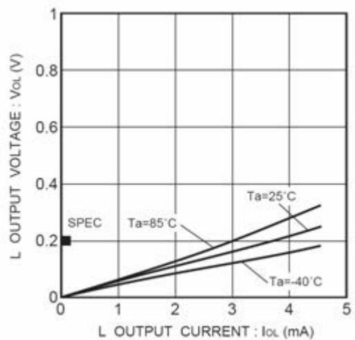
Figure 5. L output voltage  $V_{OL}$ - $I_{OL}$  ( $V_{CC}=2.5\text{V}$ )
