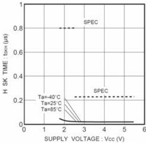
Figure 20. SK high time t<sub>SKH</sub>
