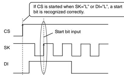
Figure 43. Normal action timing
