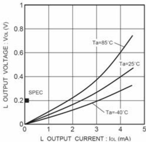
Figure 4. L output voltage  $V_{OL}$ - $I_{OL}$  ( $V_{CC}=1.8\text{V}$ )
