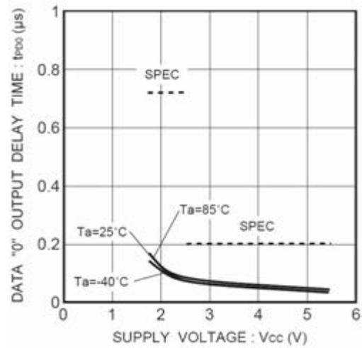
Figure 27. Data "0" output delay time  $t_{PO0}$
