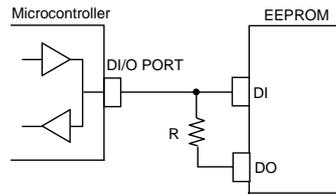
Figure 53. DI, DO control line common connection
