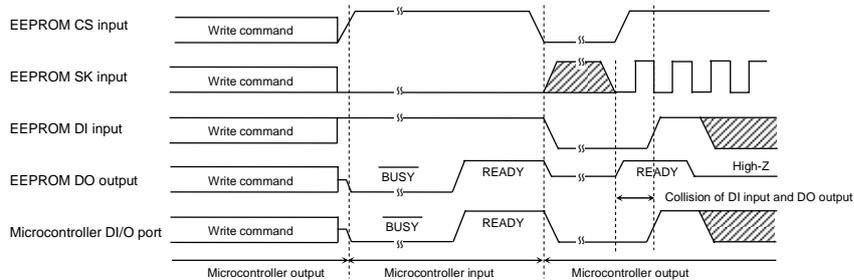
Figure 55. Collision timing at DI, DO direct connection
