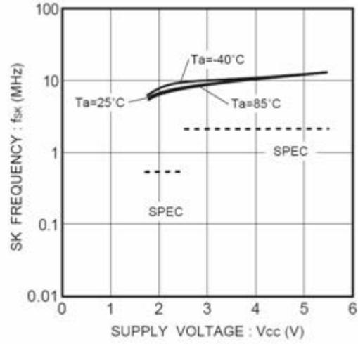
Figure 19. SK frequency f<sub>SK</sub>
