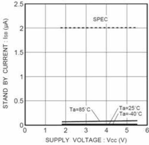
Figure 18. Consumption current at standby action I<sub>SB</sub>
