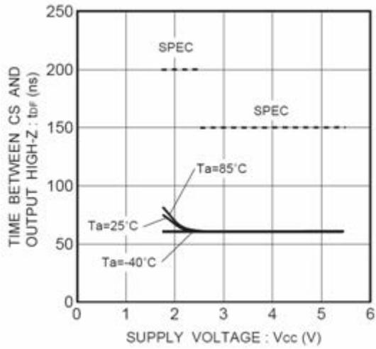
Figure 30. Time from CS to High-Z  $t_{DF}$
