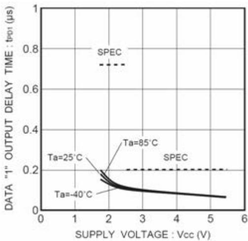
Figure 28. Output data "1" delay time  $t_{PD1}$
