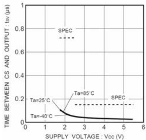
Figure 29. Time from CS to output establishment  $t_{SV}$
