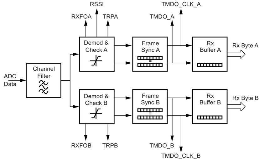
The channel filter determines the receiver bandwidth. Its output is used for both receiving paths A and B. Therefore, it has to be configured to be suitable for both. The receiving paths A and B are identical and consist of an ASK/FSK demodulator with attached signal checks, a frame synchronizer supporting pattern based search for the telegram start and a 1 byte hardware buffer for received data.
