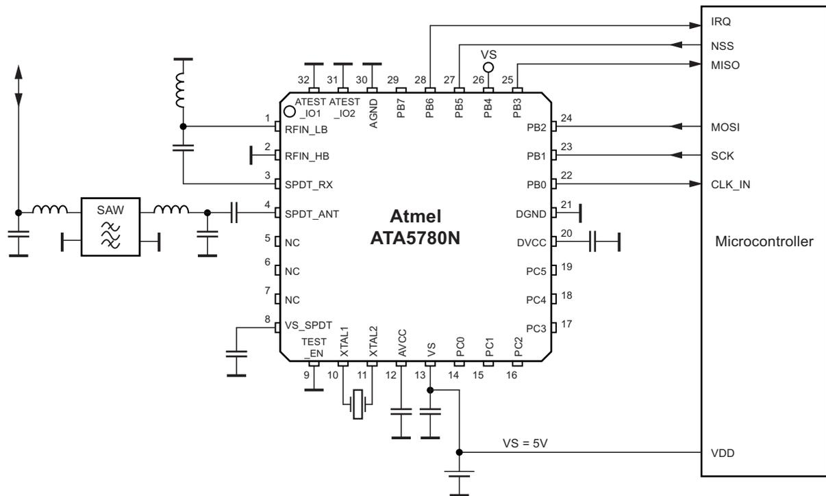
Figure 1-2 shows the typical application circuit with an external host microcontroller running from a 5V supply. For a 3V application VS and VS\_SPDT have to be shorted. The pin PB4 (PWRON) is directly connected to VS and the Atmel® ATA5780N enters the IDLEMode after power-on. The Atmel ATA5780N can work autonomously while the microcontroller stays powered down to achieve low current consumption while being sensitive to RF telegrams.
