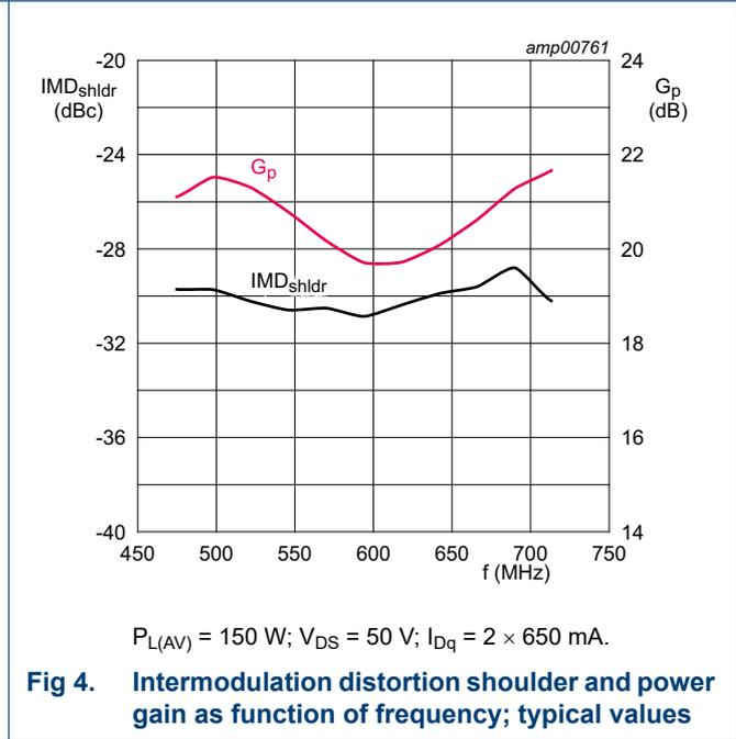
7.3.3 DVB-T performance measured in production RF test circuit
