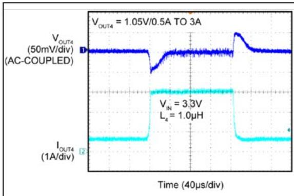
**FIGURE 2-31:** Buck 4 Load Transient – 0.5A to 3A.
