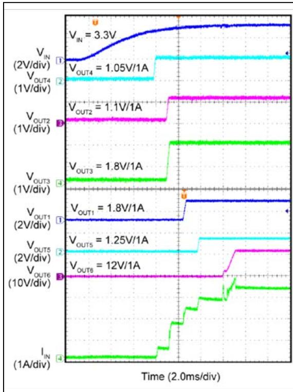
**FIGURE 2-46:** Input Supply Inrush Current – Loaded.
