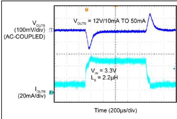
**FIGURE 2-35:** Boost 6 Load Transient – 10 mA to 50 mA.
