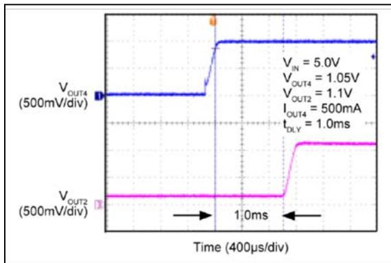
**FIGURE 2-25:** Standard Delay.
