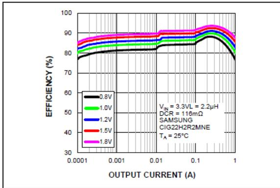
**FIGURE 2-7:** Buck Efficiency (LDCR = 116 mΩ) vs. Output Current.
