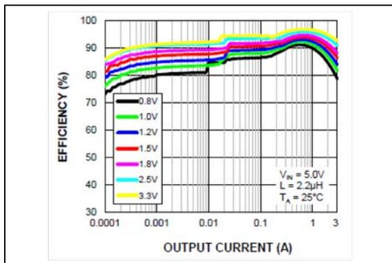
**FIGURE 2-2:** Buck Efficiency (LDCR = 0 mΩ) vs. Output Current.
