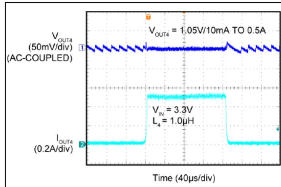
**FIGURE 2-33:** Buck 4 Load Transient – 10 mA to 0.5A.
