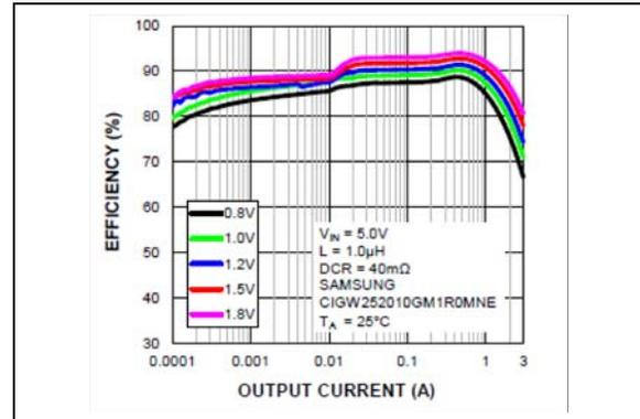
**FIGURE 2-4:** Buck Efficiency (LDCR = 40 mΩ) vs. Output Current.
