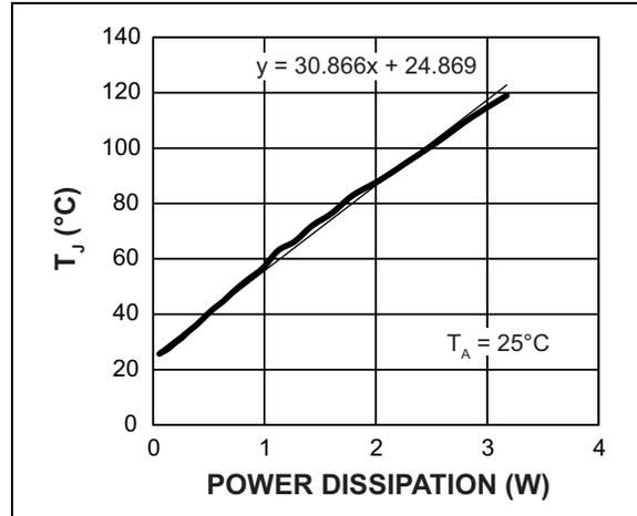
**FIGURE 4-16:** Power Dissipation.
