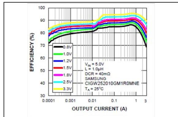
**FIGURE 2-5:** Buck Efficiency (LDCR = 40 mΩ) vs. Output Current.
