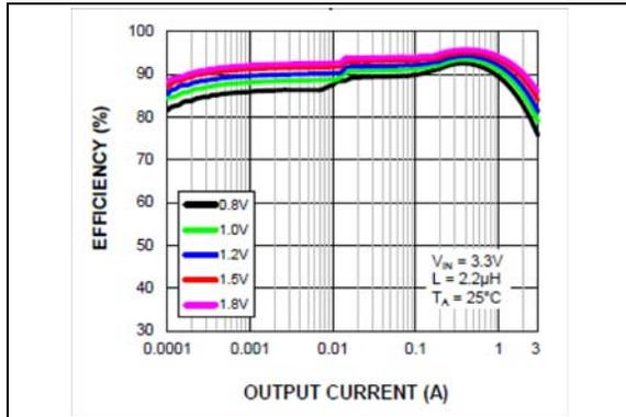
**FIGURE 2-1:** Buck Efficiency (LDCR = 0 mΩ) vs. Output Current.
