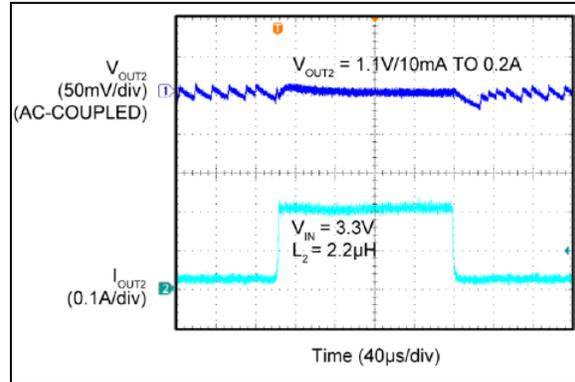
**FIGURE 2-32:** Buck 2 Load Transient – 10 mA to 0.2A.
