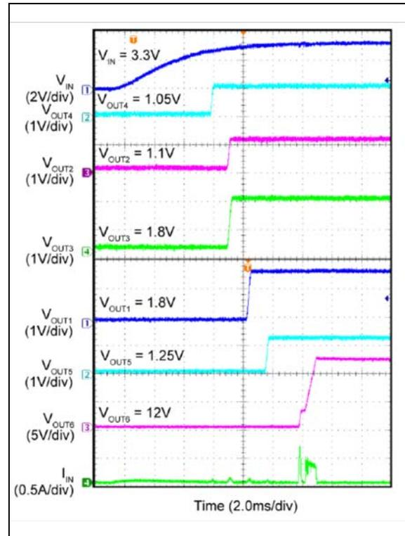
**FIGURE 2-45:** Input Supply Inrush Current – No Load.
