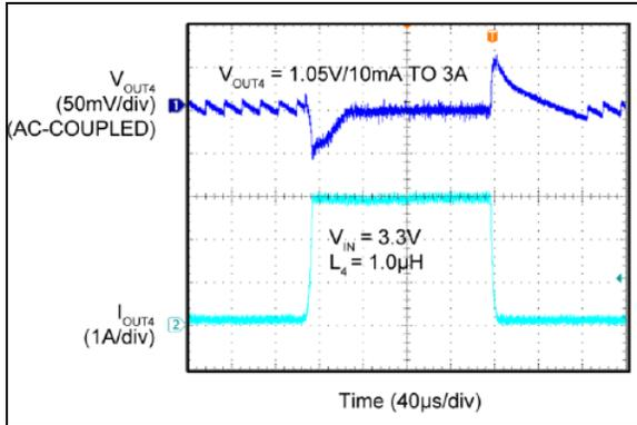
**FIGURE 2-29:** Buck 4 Load Transient – 10 mA to 3A.
