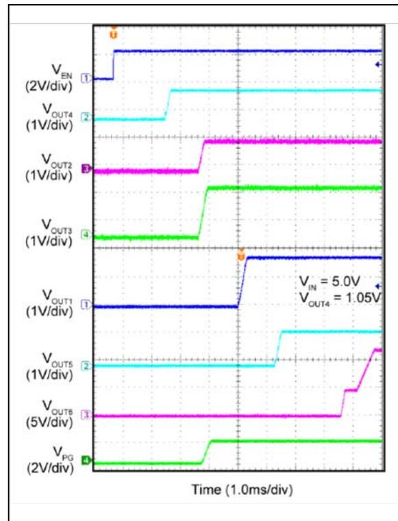
**FIGURE 2-49:** Power Good with All Outputs Masked (Mask [1-6] = 1).
