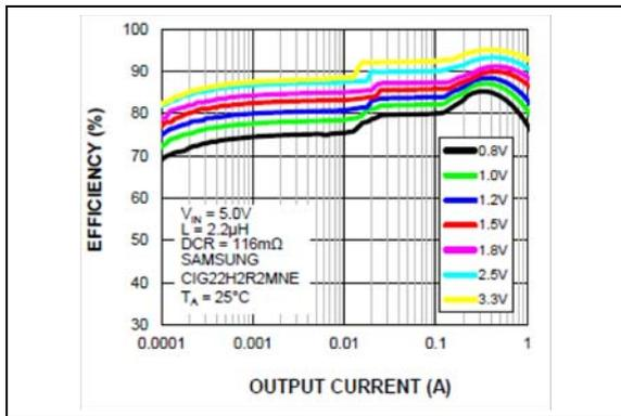
**FIGURE 2-8:** Buck Efficiency (LDCR = 116 mΩ) vs. Output Current.
