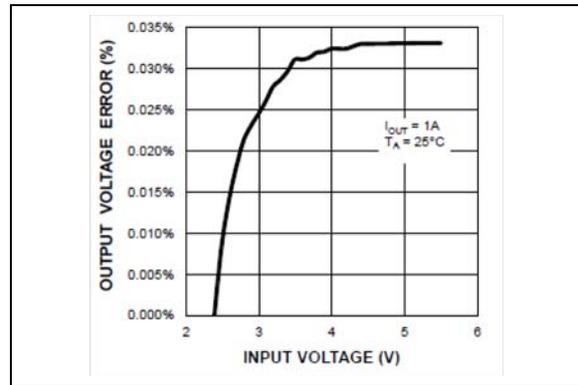
**FIGURE 2-12:** Buck Line Regulation vs. Input Voltage.
