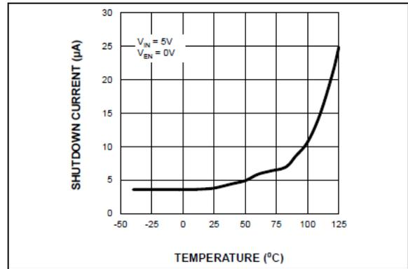
**FIGURE 2-16:**  $V_{IN}$  Shutdown Supply Current vs. Temperature.
