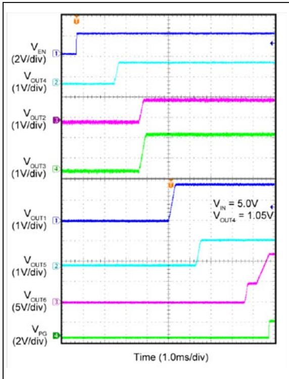
**FIGURE 2-50:** Power Good with All Outputs Masked except V<sub>OUT6</sub> (Mask [1-5] = 1; Mask [6] = 0).
