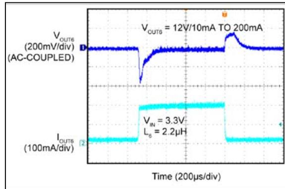
**FIGURE 2-34:** Boost 6 Load Transient – 10 mA to 200 mA.
