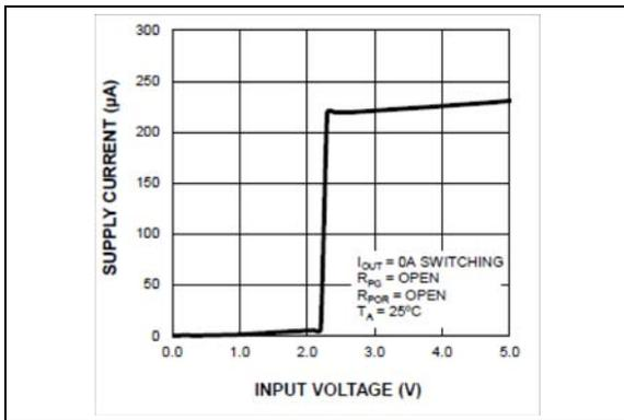
**FIGURE 2-14:**  $V_{IN}$  Operating Supply Current vs. Input Voltage.
