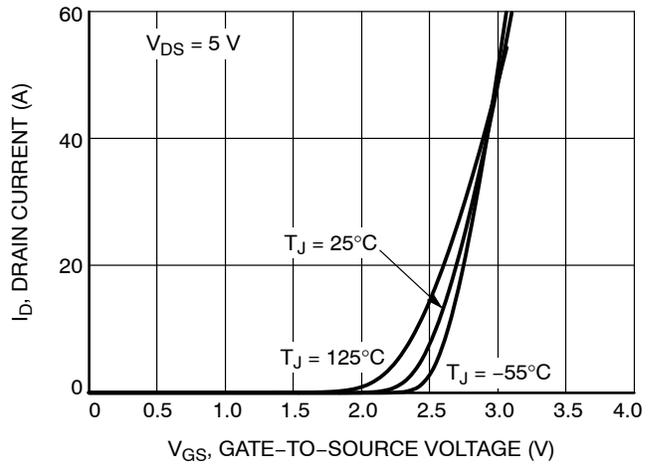
Figure 2. Transfer Characteristics
