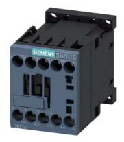
Power contactor, AC-3 9 A, 4 kW / 400 V 1 NO, 100 V AC, 50 Hz 100-110 V, 60 Hz, 3-pole Size S00, screw terminal
