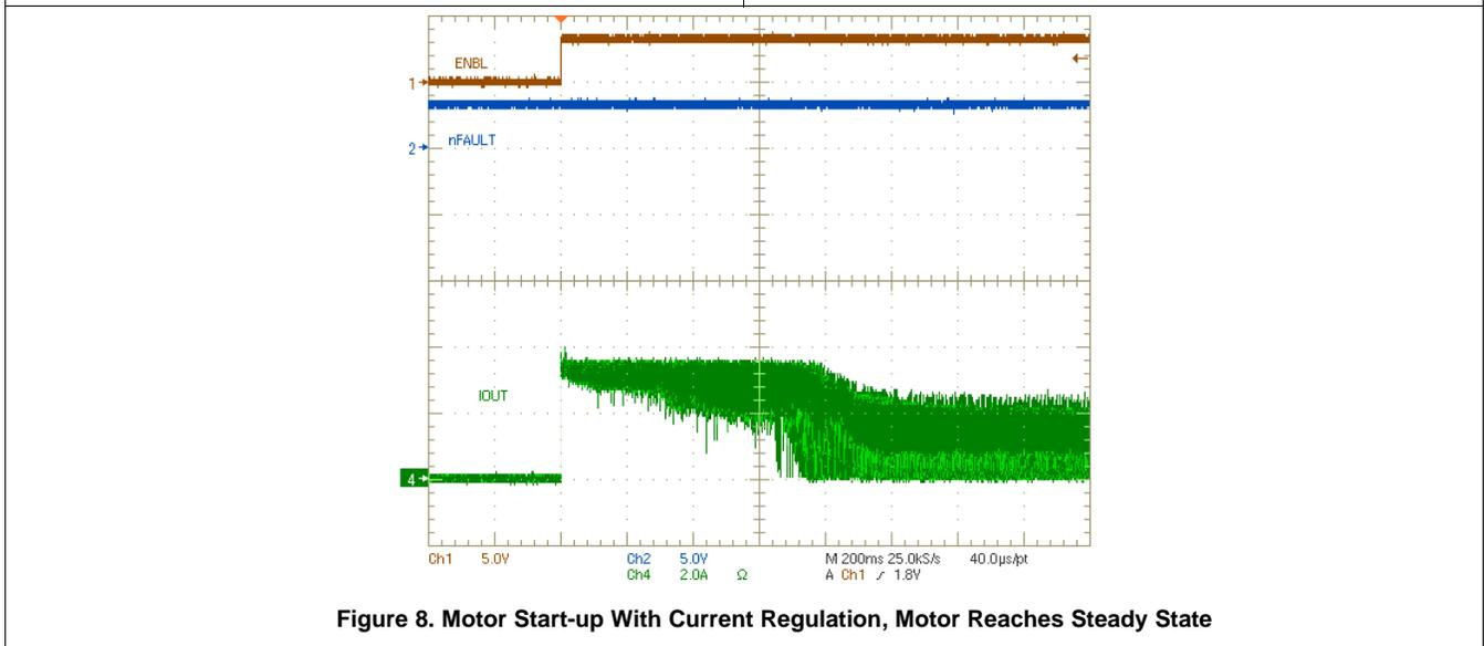
Figure 8. Motor Start-up With Current Regulation, Motor Reaches Steady State
