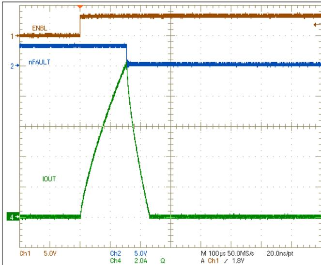
Figure 6. Motor Start-up without Current Regulation, Overcurrent Trips
