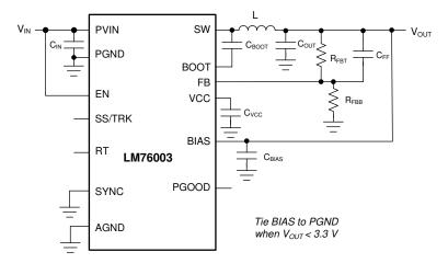
Figure 21. LM76002/LM76003 Basic Schematic
