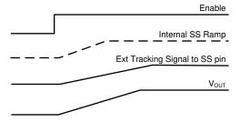
Figure 15. Tracking With Longer Start-up Time Than The Internal Ramp
