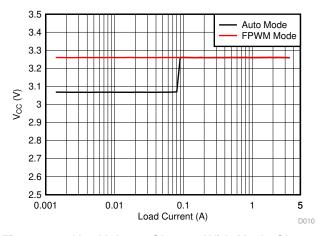
Figure 13. V<sub>CC</sub> Voltage Change With Mode Change
