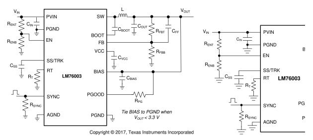
Figure 22. LM76002/LM76003 Comprehensive Schematic
