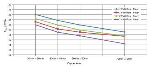
Figure 86. Measured  $R_{\theta JA}$  vs PCB Copper Area on a 2-Layer Board and a 4-Layer Board
