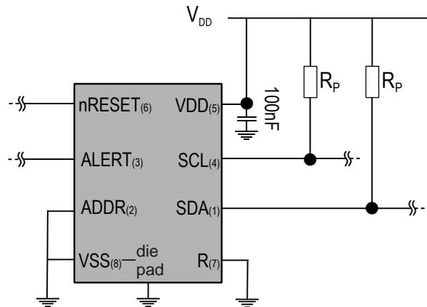
**Figure 3.** Typical application circuit. Please note that the positioning of the pins does not reflect the position on the real sensor (see **Table 8**).
