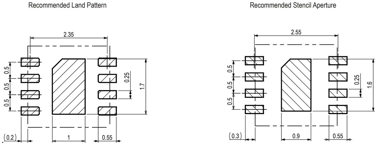
**Figure 7.** Recommended metal land pattern (left) and stencil apertures (right) for SHT33-DIS. The dashed lines represent the outer dimension of the DFN package. The PCB pads (left) and stencil apertures (right) are indicated through the shaded areas.
