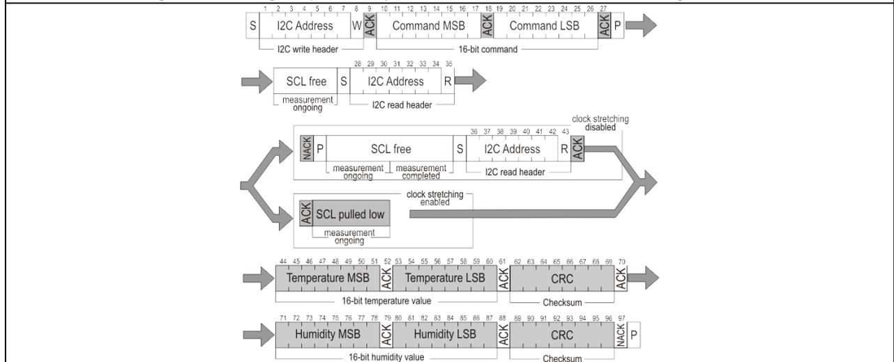
**Table 10.** Measurement commands in single shot mode. The first “SCL free” block indicates a minimal waiting time of 1 ms. (Clear blocks are controlled by the microcontroller, grey blocks by the sensor).
