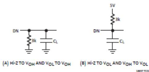
Load Circuits for Output Float Delay
