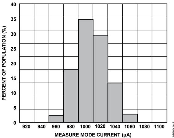
Figure 12. Measure Mode Current Histogram at 25°C
