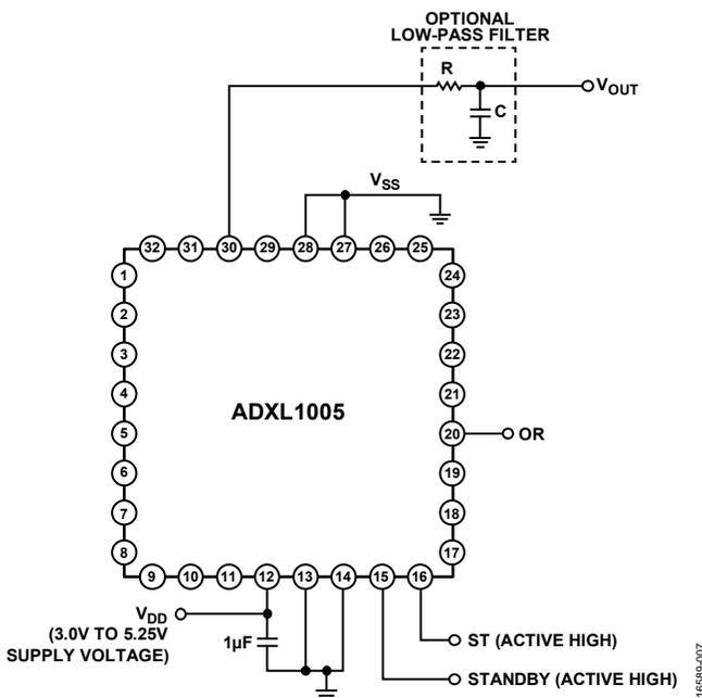
Figure 20. Application Circuit
