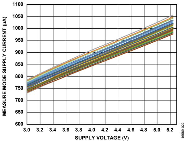
Figure 11. Measure Mode Supply Current vs. Supply Voltage
