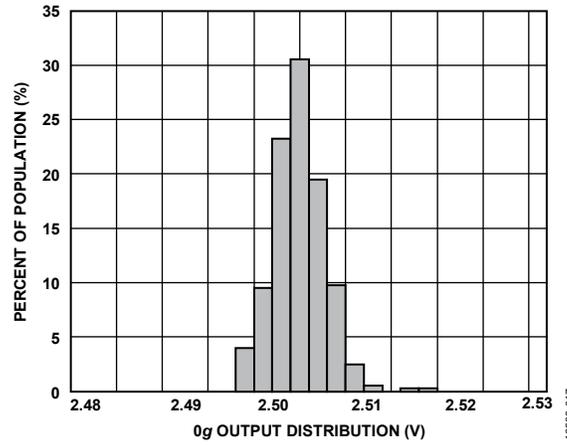
Figure 13. 0 g Offset Histogram at 25°C
