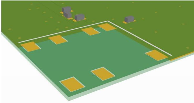
The clear-out area is simply defined as the same size as the antenna. No additional clearance is required.
