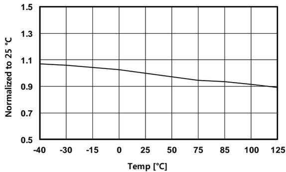
Figure 9. f<sub>MAX-CC</sub> vs. Temperature
