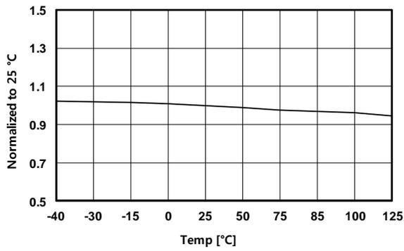
Figure 5. V<sub>DD-ON</sub> vs. Temperature
