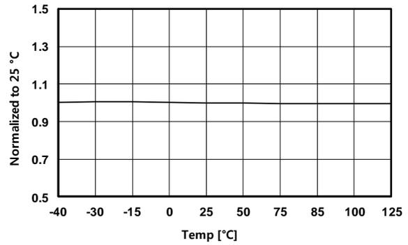
Figure 8. V<sub>OV</sub> vs. Temperature
