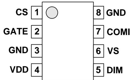
Figure 4. Pin Configuration
