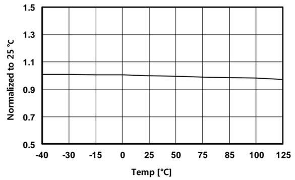
Figure 6. V<sub>DD-OFF</sub> vs. Temperature
