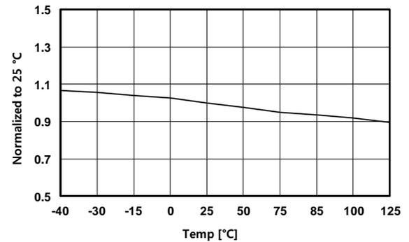
Figure 10. f<sub>MIN-CC</sub> vs. Temperature
