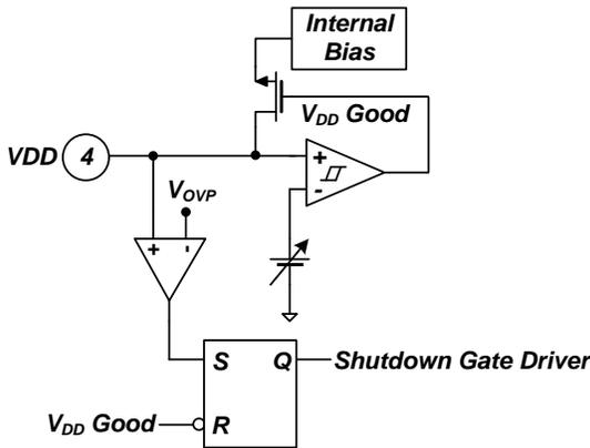
Figure 24. Internal OVP Block
