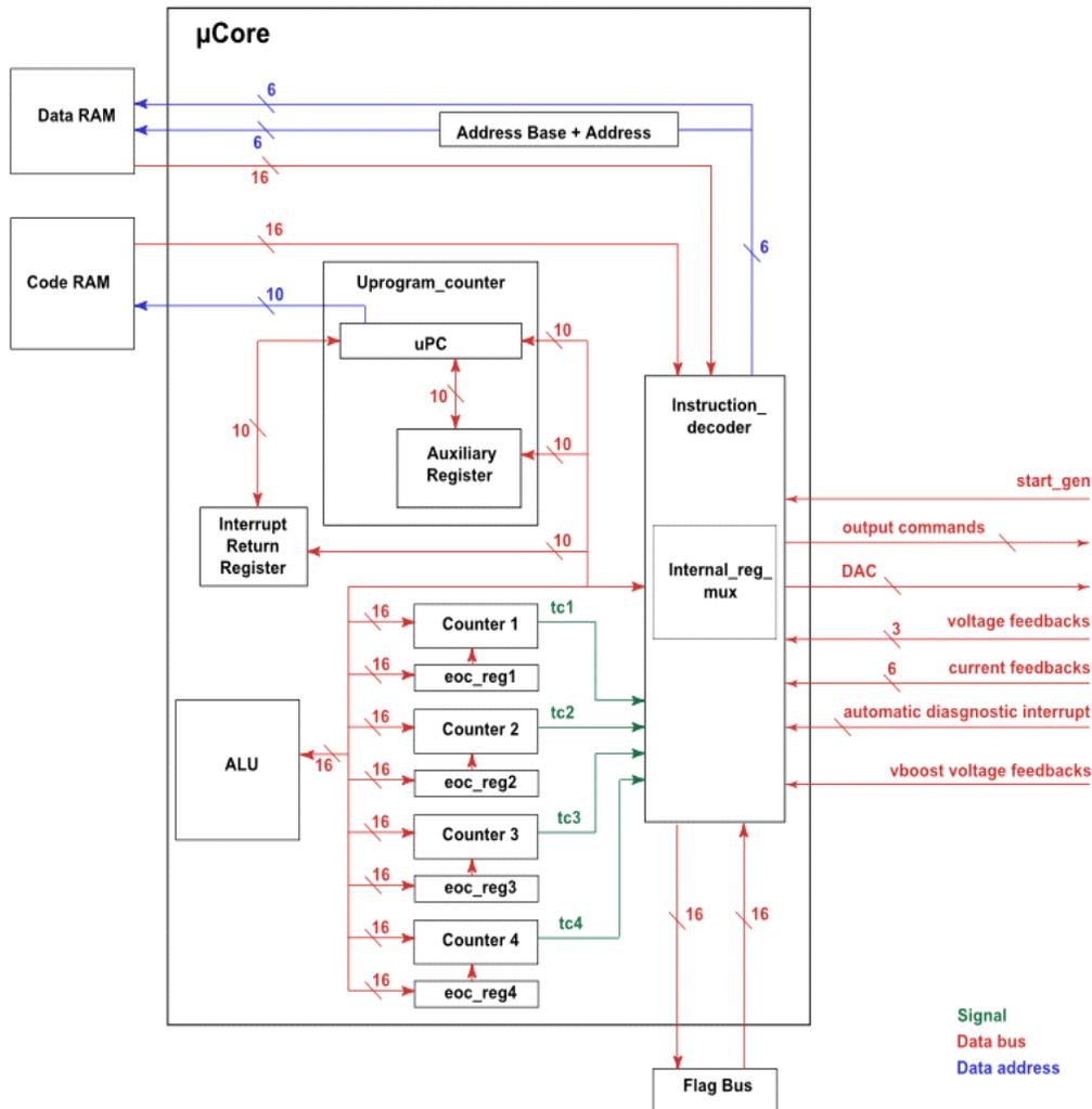
Figure 36. Microcore block diagram
