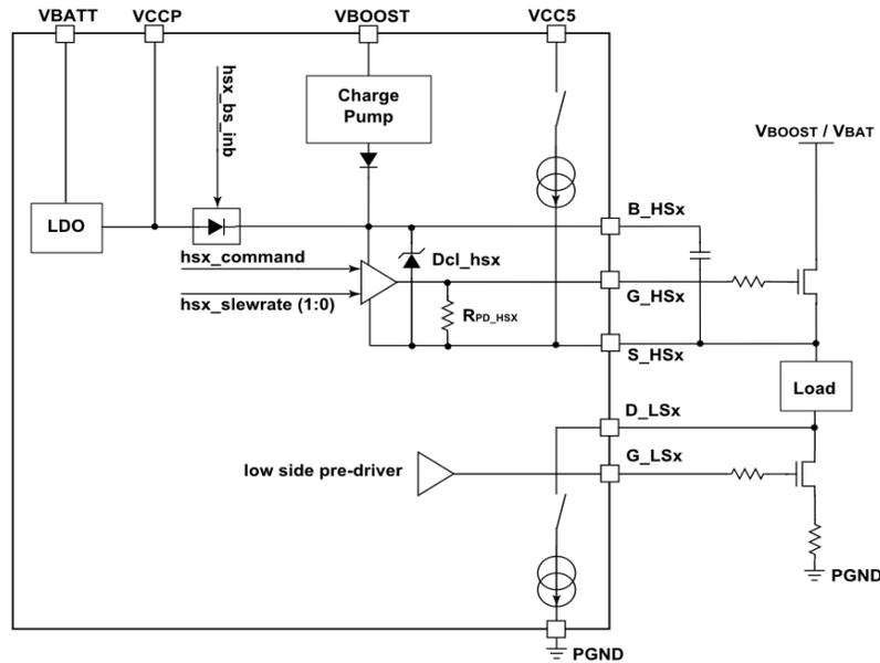
**Figure 13. High-side pre-driver block diagram**
