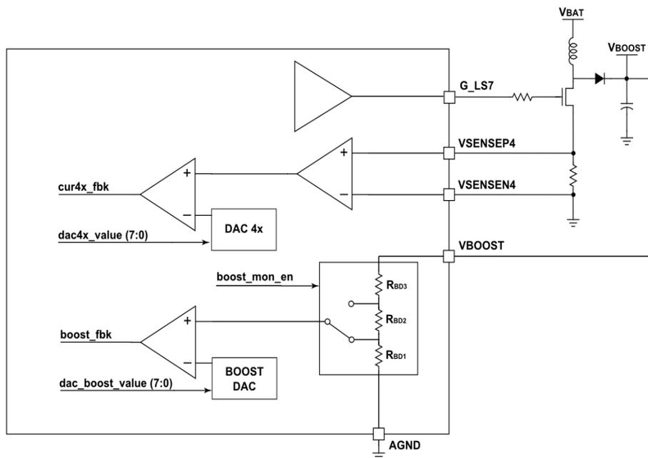
**Figure 11. Boost converter topology for fixed frequency mode**
