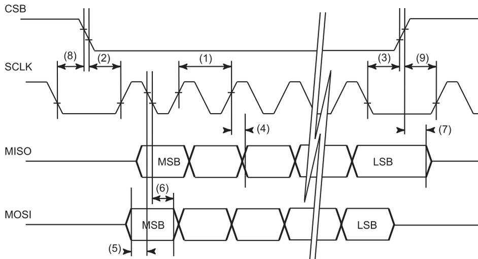
Figure 25. SPI timing
