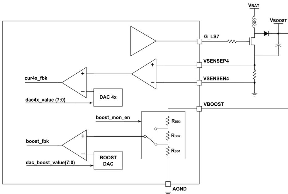
**Figure 12. Boost converter topology for variable frequency mode**
