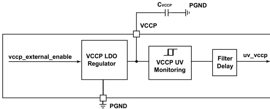
**Figure 10. V<sub>CCP</sub> undervoltage monitoring**
