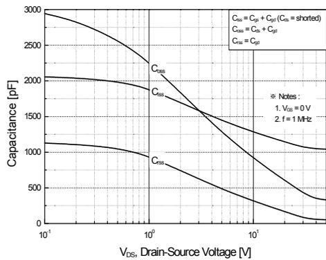
**Figure 5. Capacitance Characteristics**
