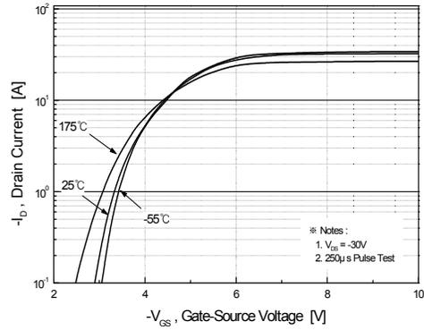
**Figure 2. Transfer Characteristics**
