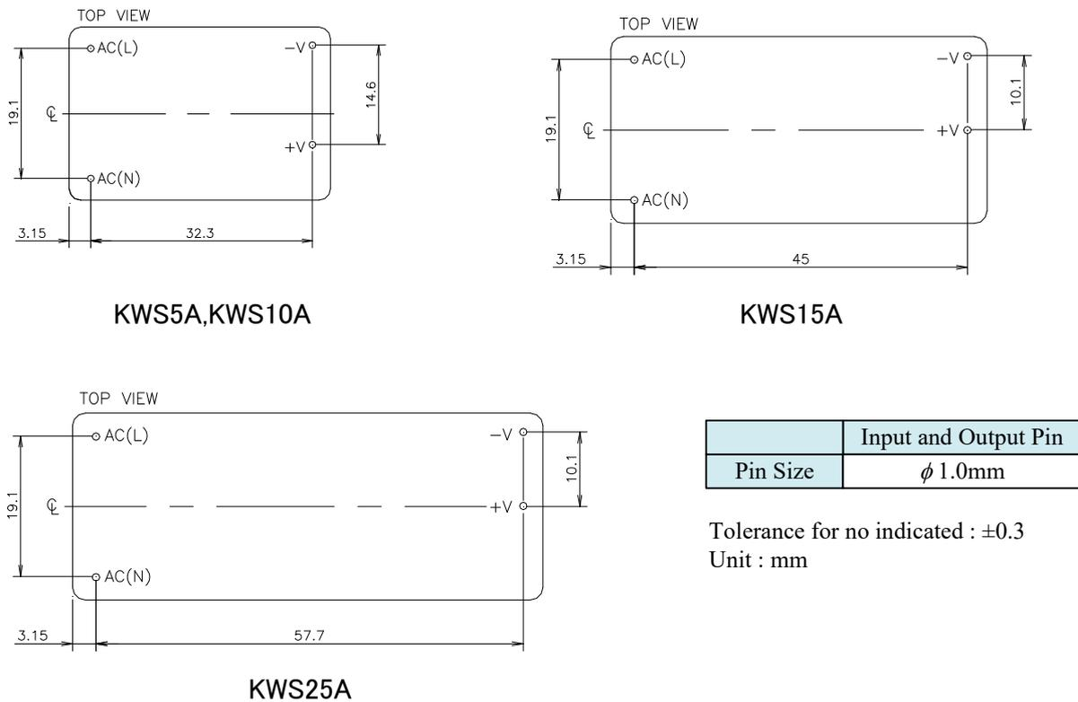
Fig.7-1 The mounting hole position
