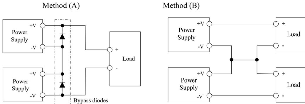
Note : In case of method (A), connect bypass diodes. If not, the unit might cause damage.
