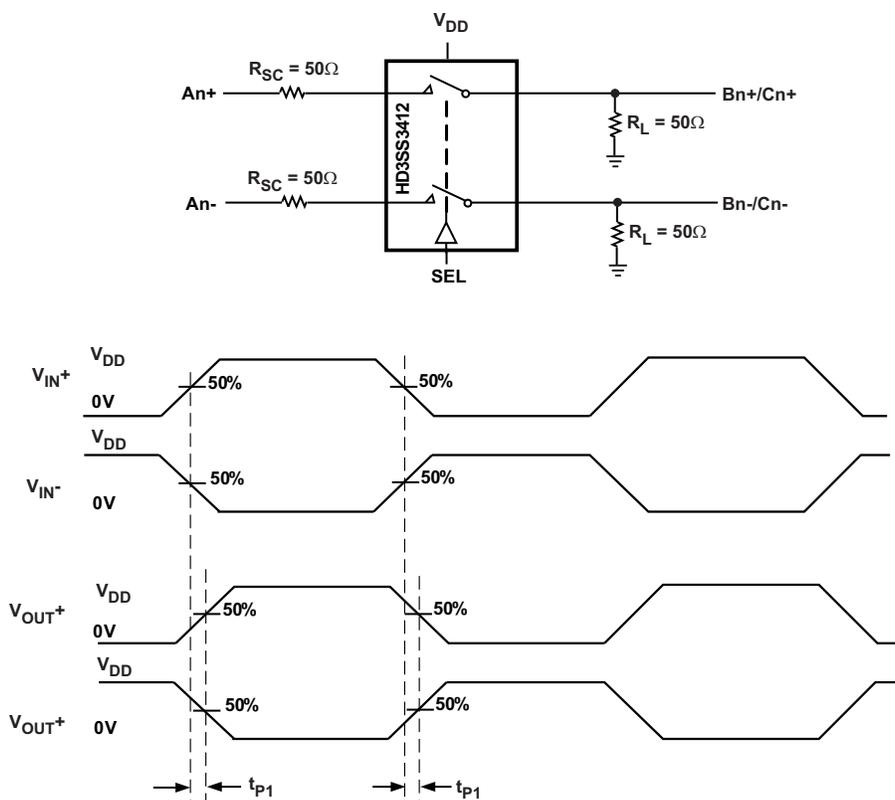
$T_{\text{SKEWInter}}$  = Difference between  $t_{\text{PD}}$  for any two pairs of outputs
