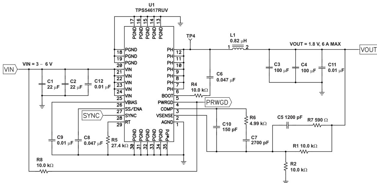
Analog and power grounds are tied at the pad under the package of the IC
