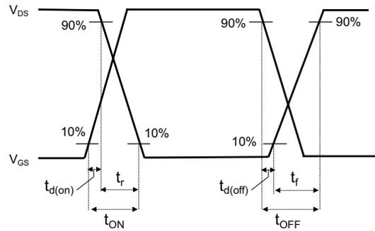
**Fig. 21. Switching time definition**
