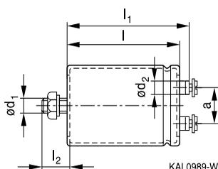
For types with threaded stud and  $d \leq 76$  mm the base is not insulated. Also refer to the mounting instructions in chapter "Capacitors with screw terminals – Accessories".
