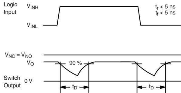
Figure 2. Break-Before-Make Interval
