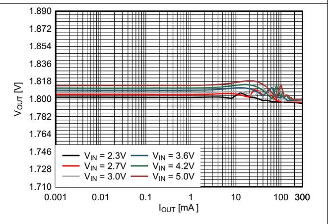
Figure 11. Output Voltage vs Output Current,  $V_{OUT} = 1.8V$
