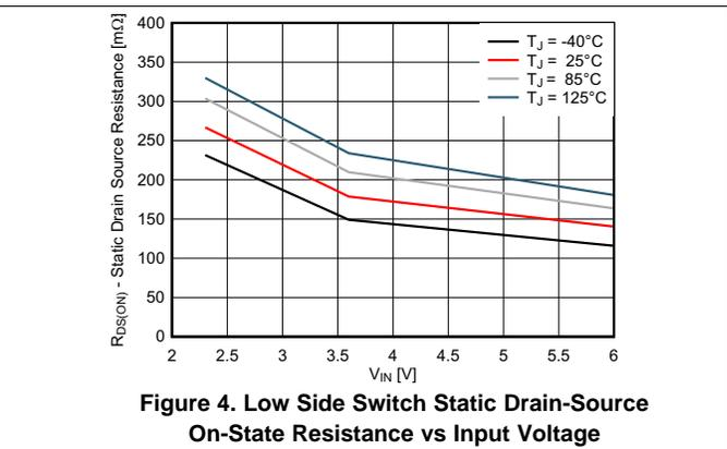
Figure 4. Low Side Switch Static Drain-Source On-State Resistance vs Input Voltage
