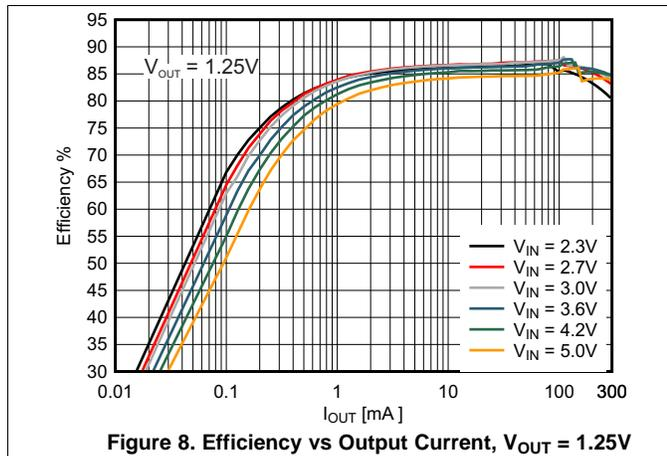
Figure 8. Efficiency vs Output Current,  $V_{OUT} = 1.25V$
