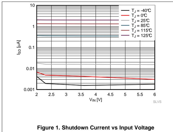
Figure 1. Shutdown Current vs Input Voltage
