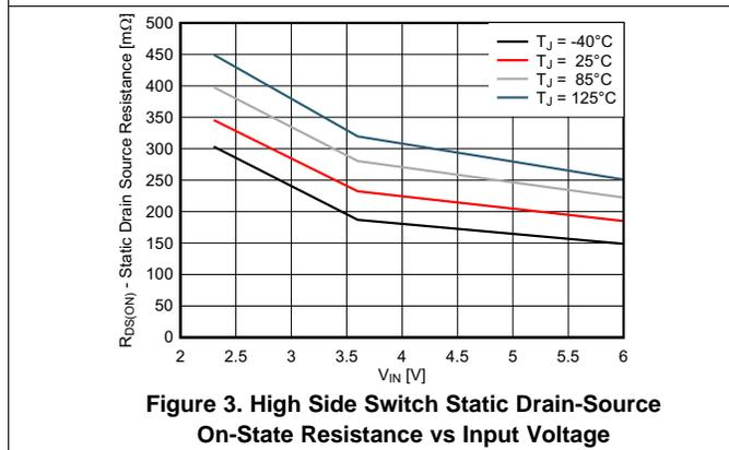
Figure 3. High Side Switch Static Drain-Source On-State Resistance vs Input Voltage
