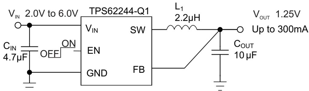
**Figure 6. TPS62244Q1, Fixed 1.25 V  $V_{OUT}$**
