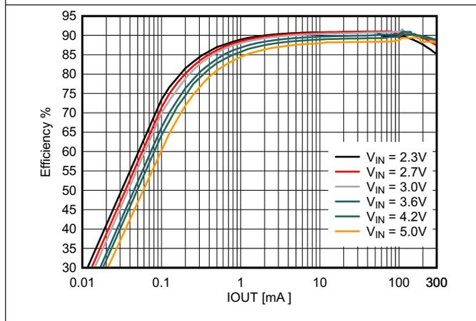
Figure 10. Efficiency vs Output Current,  $V_{OUT} = 1.8V$
