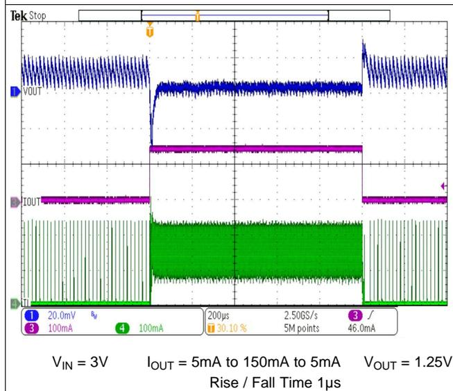
**Figure 16. Load Transient PFM / PWM Mode**
