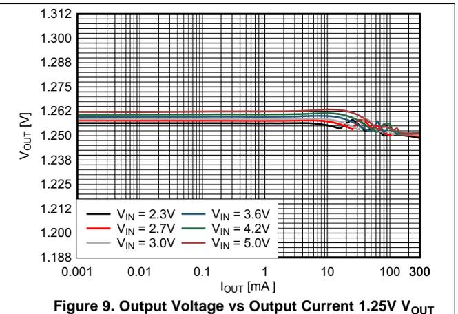
Figure 9. Output Voltage vs Output Current 1.25V  $V_{OUT}$
