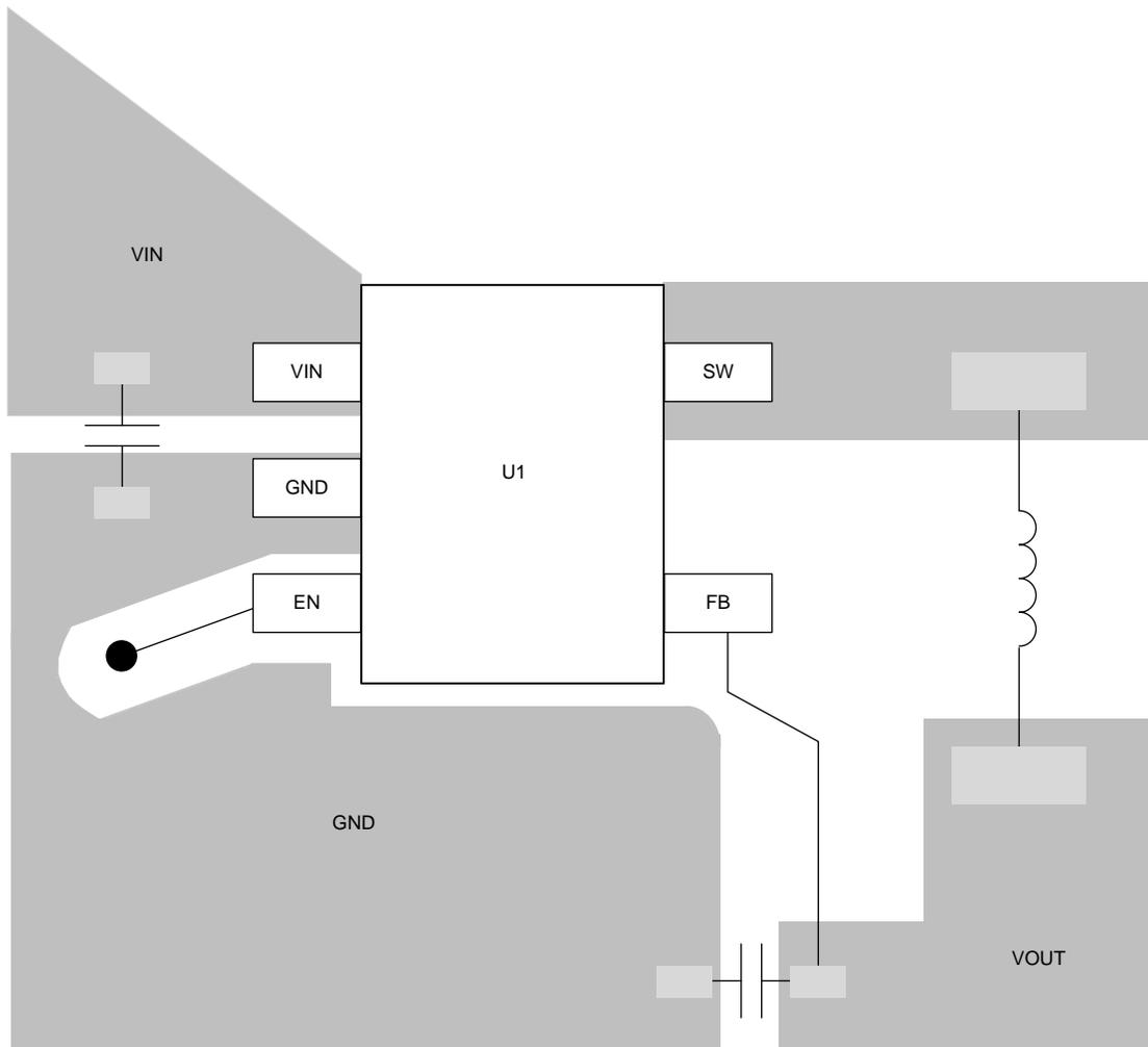
**Figure 18. Suggested Layout for Fixed Output Voltage**
