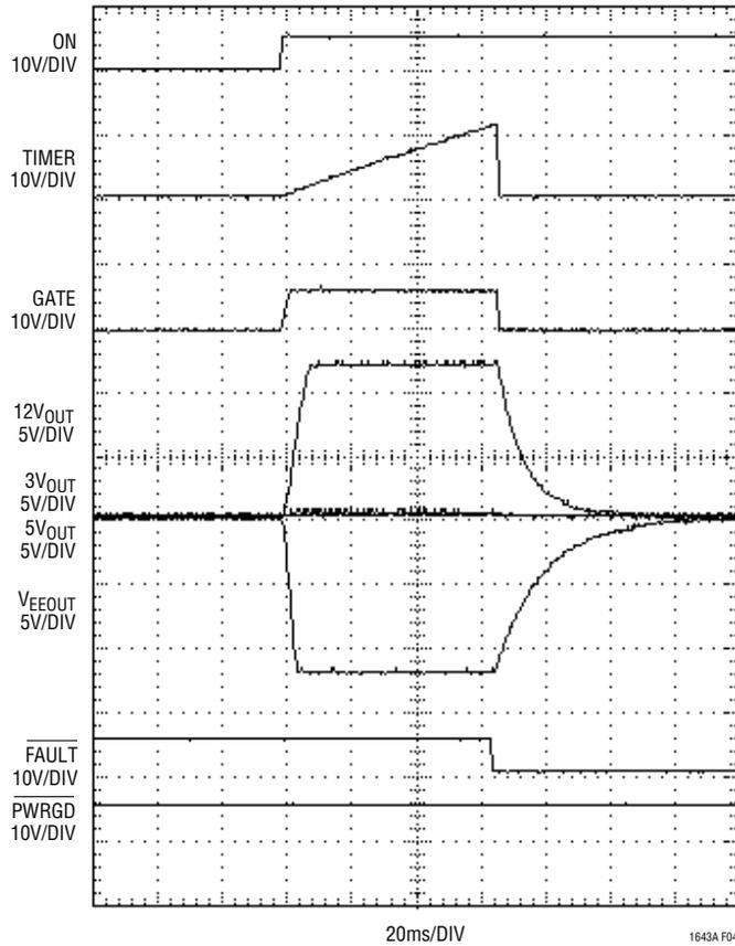
Figure 4. Power-Up into a Short on 3.3V Output
