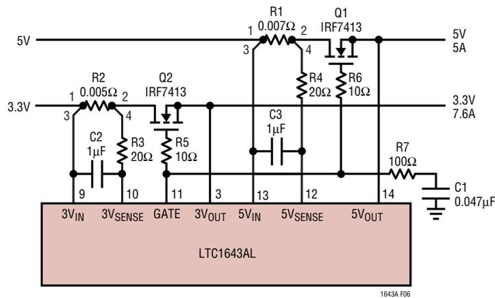
Figure 6. Delay in the Current Limit Loop
