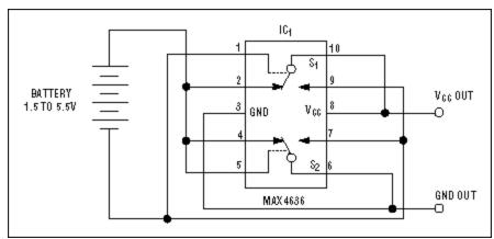
Figure 1. This circuit senses battery polarity and then quickly connects the load or swaps the battery leads.
