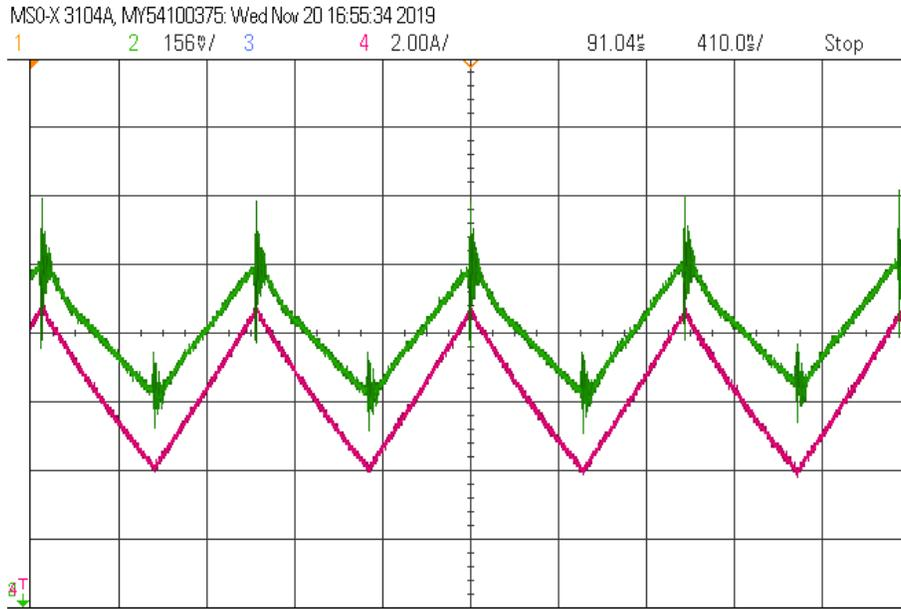
Figure 6. 1 MHz converter response. Green Trace: DS.10.2S with no output filtering. Red trace: TEKTRONIX TCP305A current probe response.
