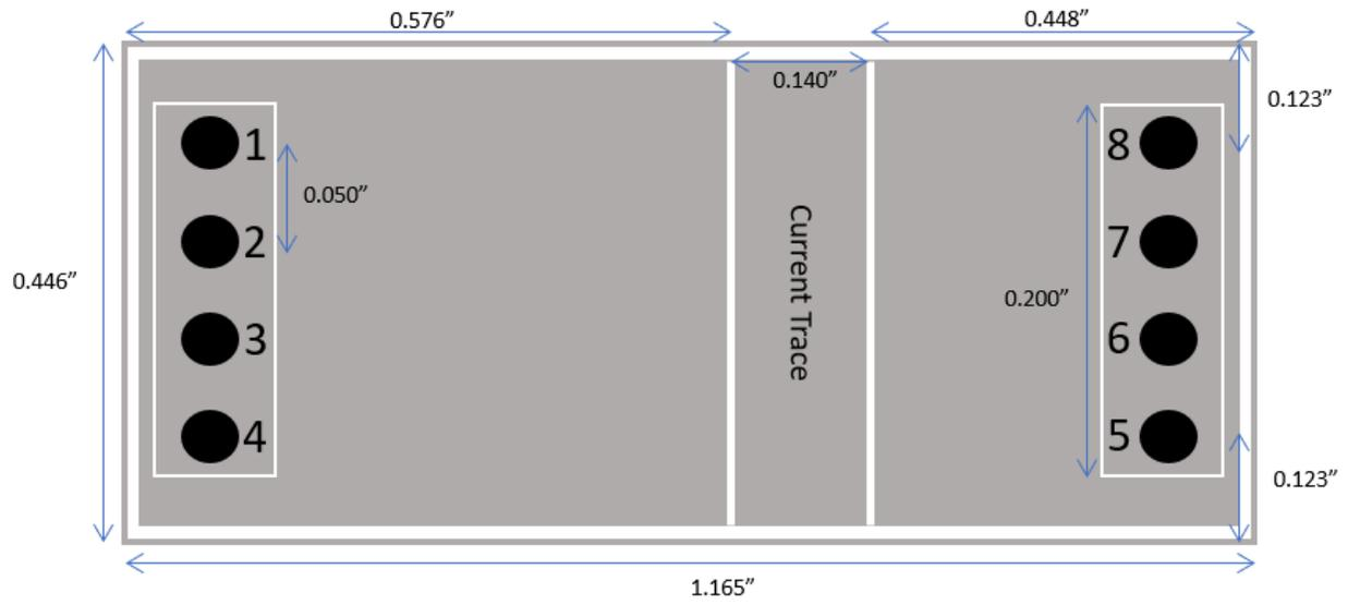
Figure 8 – Sensor Package Dimensions (Bottom View)
