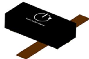
Figure 1 - Placement of contactless sensor above current trace
