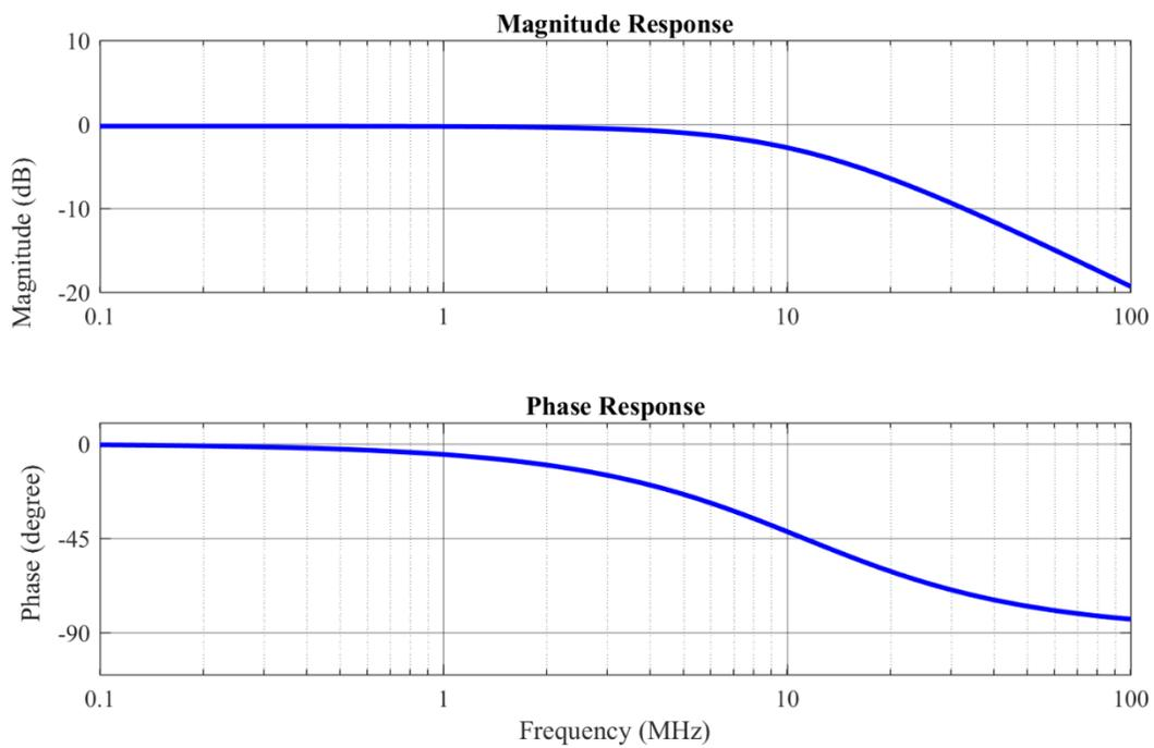
Figure 3. Frequency Response of Sensor (10MHz -3dB bandwidth)
