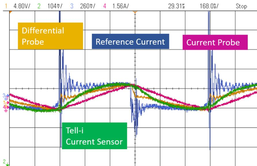
Figure 5 - Sensor operation in 1MHz switching converter with minimal inductor
