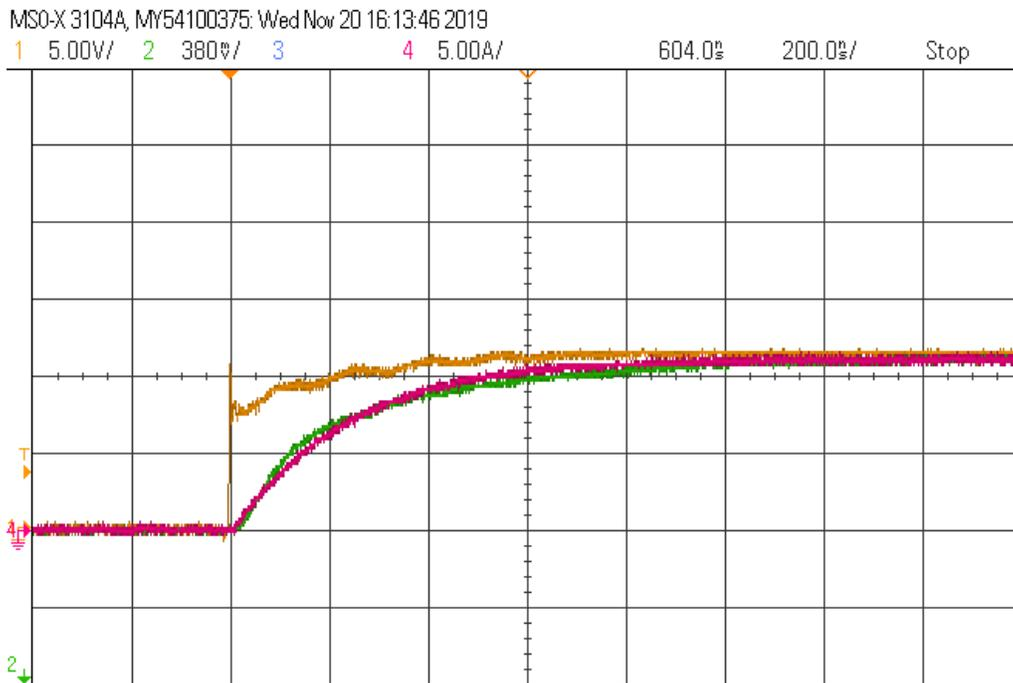
Figure 2 – Sensor response to step change in current (close view) with response and rise times shown. Green trace is the Tell-i sensor response; Red trace is the TEKTRONIX TCP305A current probe with 50 Mhz bandwidth; Orange is the reference current.
