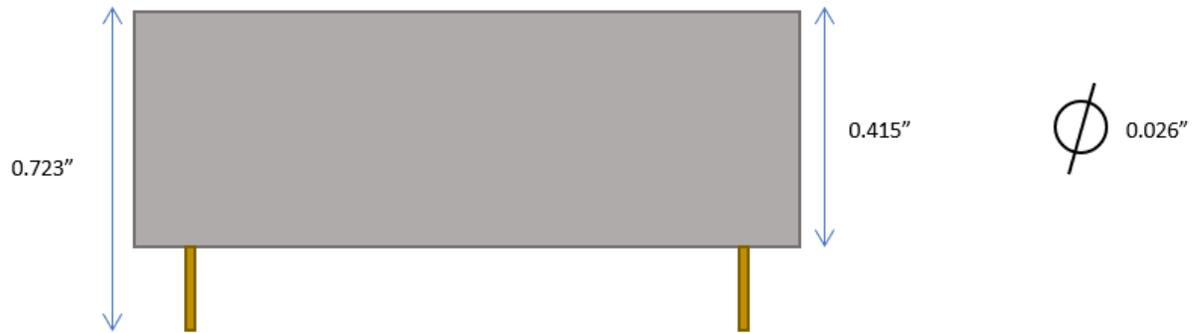
Figure 8 -Height Dimensions and Pin Hole Size
