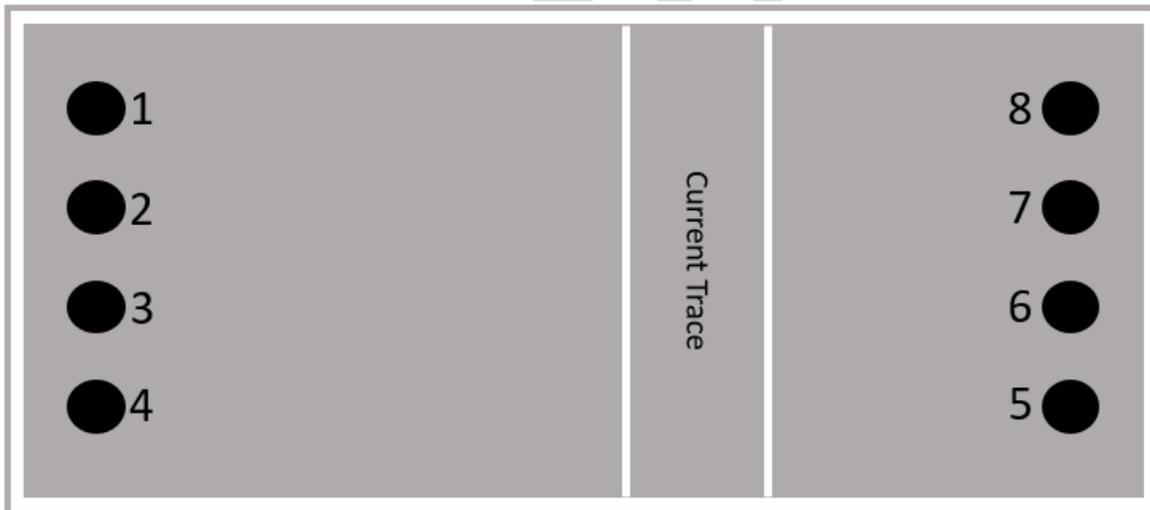
Figure 7 - Pinout Diagram (Bottom View)
