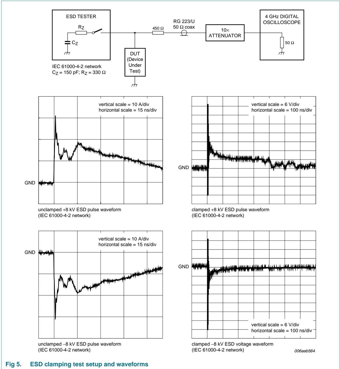
**Fig 5. ESD clamping test setup and waveforms**
