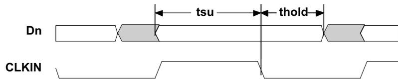
All input timing is defined at  $IOVDD / 2$  on an input signal with a 10% to 90% rise or fall time of less than 3 ns. CLKSEL = 0V.
