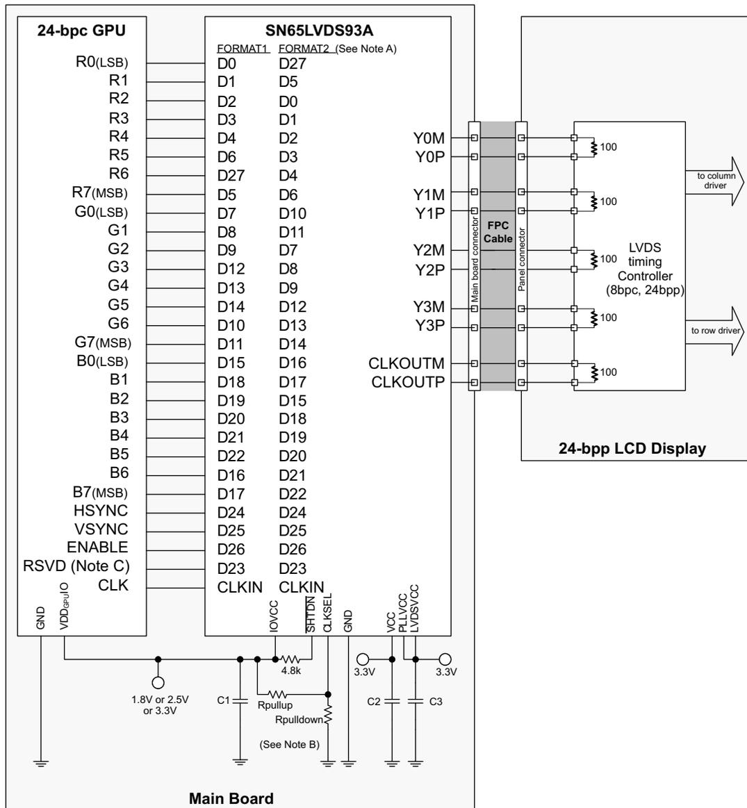
Note A. **FORMAT:** The majority of 24-bit LCD display panels require the two most significant bits (2 MSB ) of each color to be transferred over the 4th serial data output Y3. A few 24-bit LCD display panels require the two LSBs of each color to be transmitted over the Y3 output. The system designer needs to verify which format is expected by checking the LCD display data sheet.
