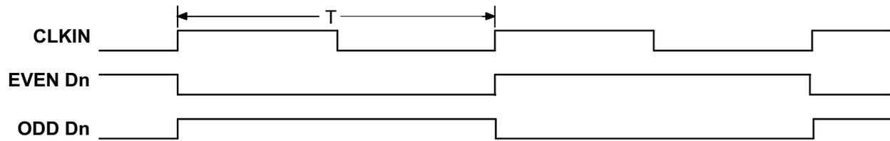
The worst-case test pattern produces nearly the maximum switching frequency for all of the LVDS outputs.
