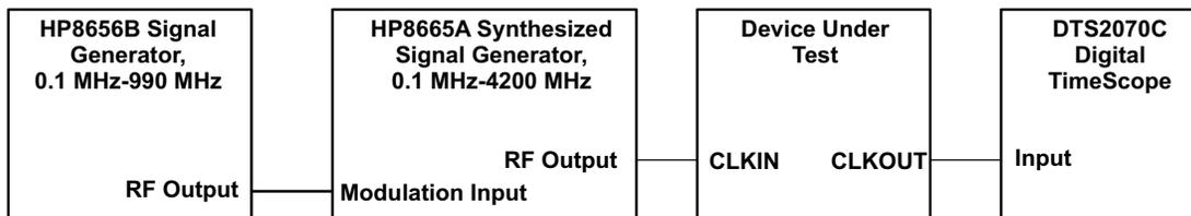
Figure 11. Output Clock Jitter Test Set Up
