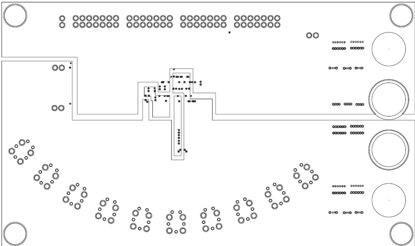
**Figure 25. SN65LVDS93A EVM VCC Layer – TSSOP Package**
