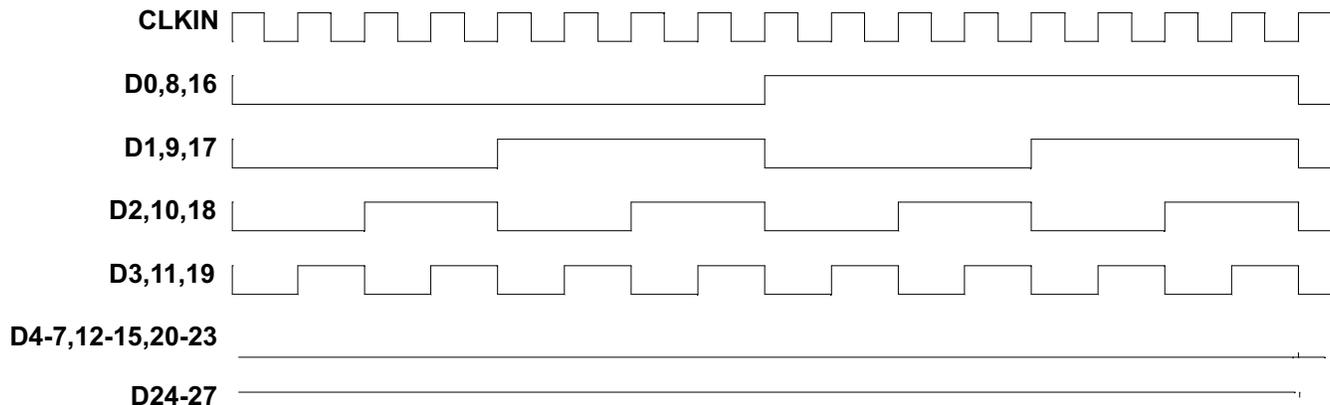
The 16 grayscale test pattern test device power consumption for a typical display pattern.
