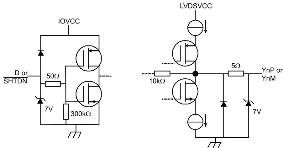
**Figure 5. Equivalent Input and Output Schematic Diagrams**
