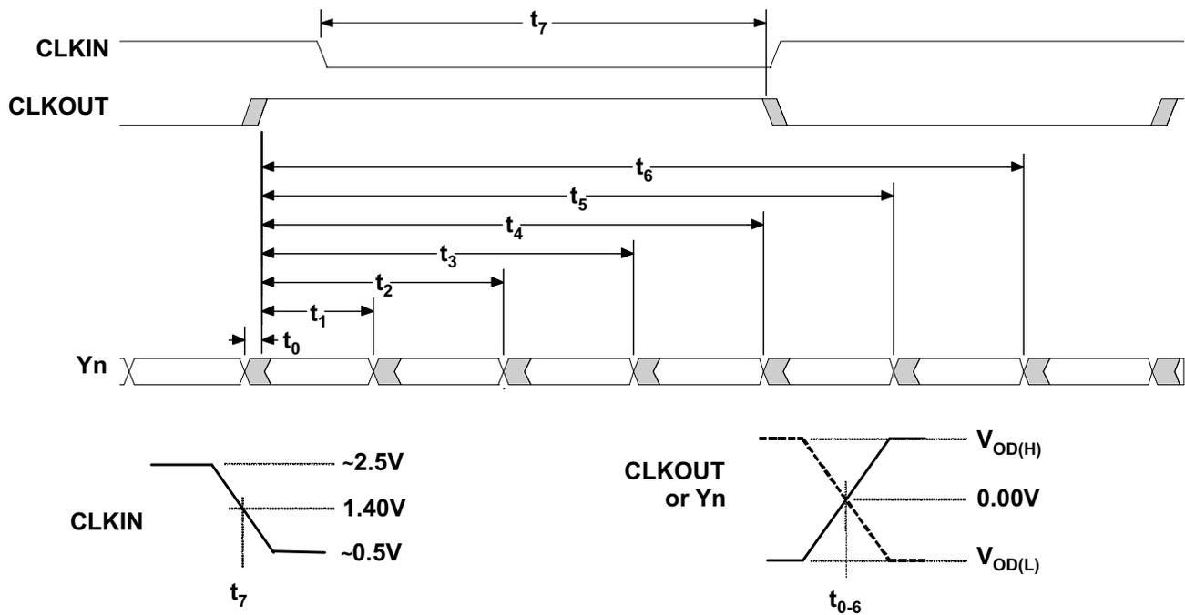
CLKOUT is shown with CLKSEL at high-level.
