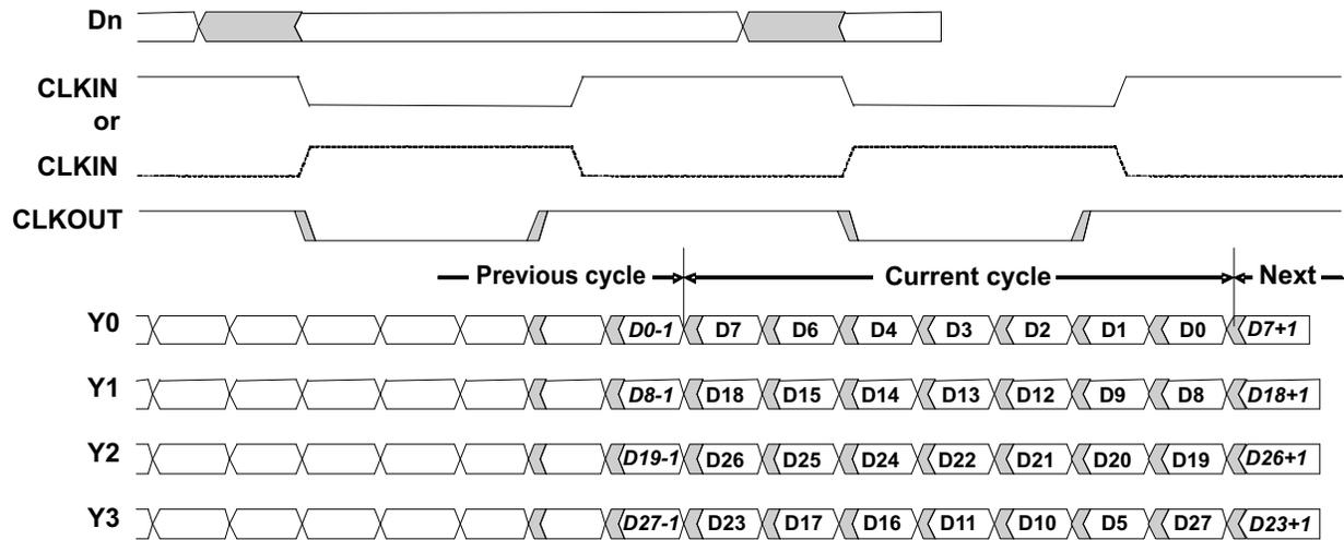
**Figure 1. Typical SN65LVDS93A Load and Shift Sequences**
