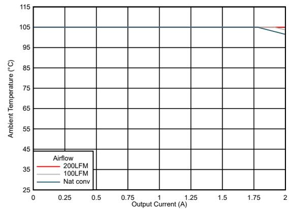
Figure 7-14. Safe Operating Area ( $V_{OUT} = 3.3\text{ V}$ )
