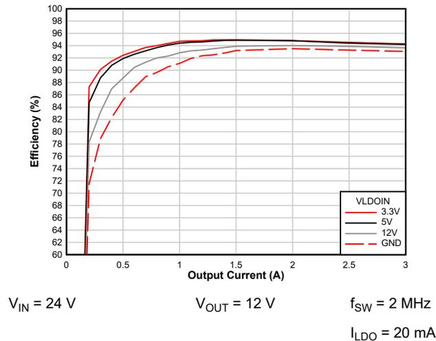
**Figure 8-9. Efficiency Improvements with VLDOIN ( $V_{OUT} = 12\text{ V}$ )**
