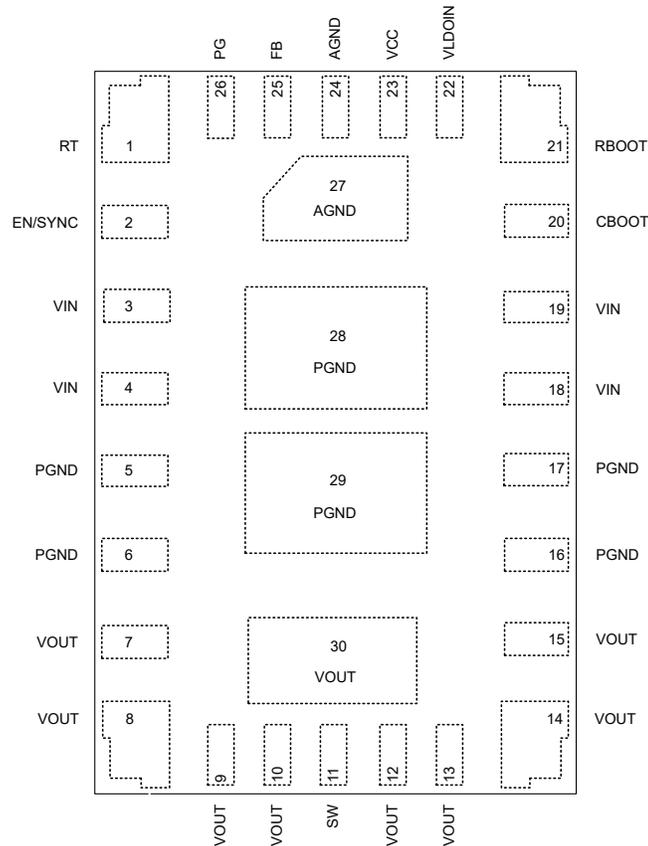
Figure 6-1. 30-Pin QFN, RDH Package (Top View)
