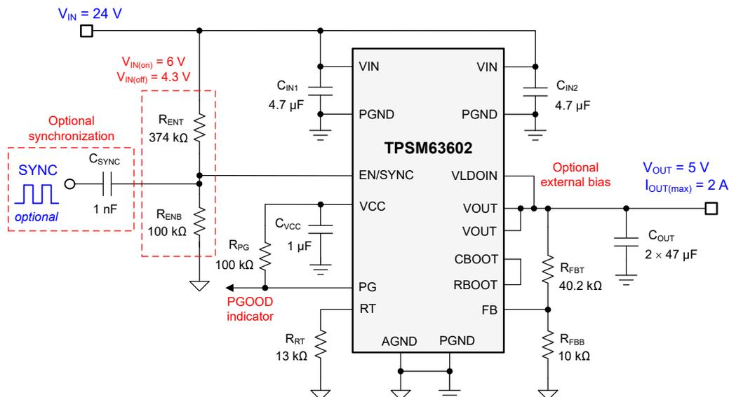
Figure 9-1. Circuit Schematic
