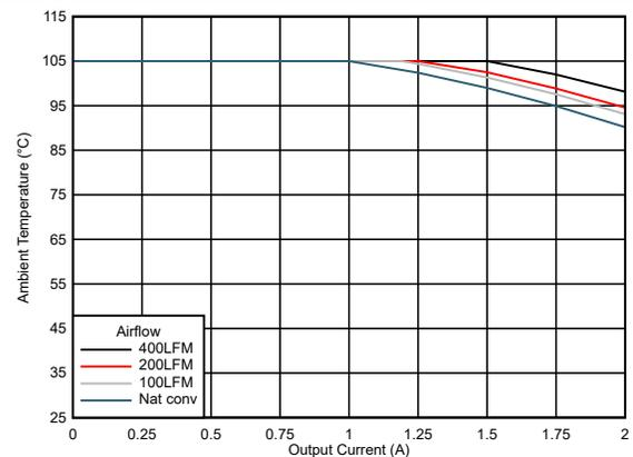
Figure 7-16. Safe Operating Area ( $V_{OUT} = 12\text{ V}$ )
