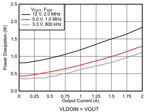
Figure 7-18. Power Dissipation
