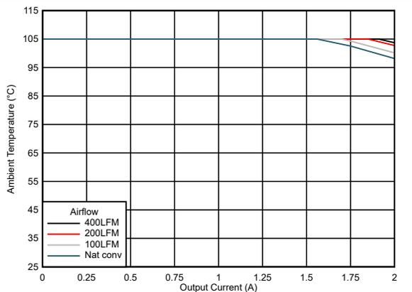
Figure 7-15. Safe Operating Area ( $V_{OUT} = 5.0\text{ V}$ )
