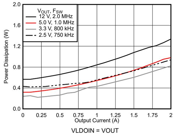
Figure 7-12. Power Dissipation
