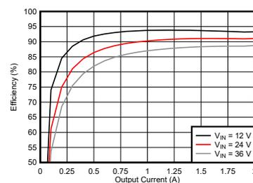
**Typical Efficiency, V<sub>OUT</sub> = 5 V, f<sub>sw</sub> = 1 MHz**
